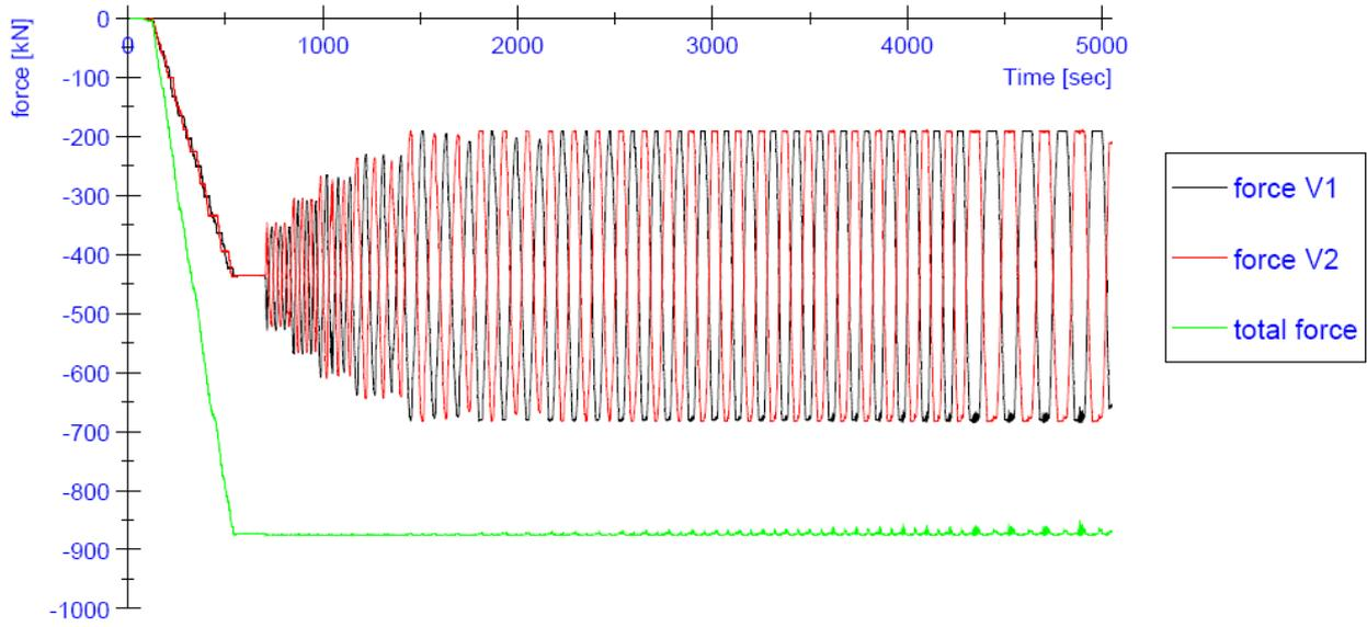
**Figure 96:** Progress of the vertical forces V1 and V2 during the test on specimen CS07
