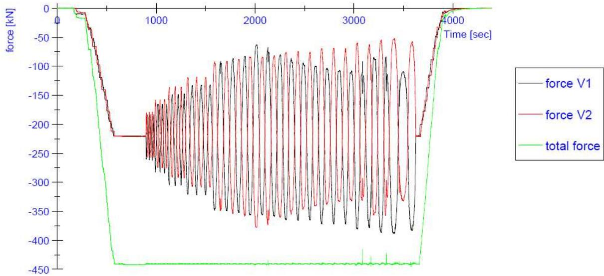
**Figure 48:** Progress of the vertical forces V1 and V2 during the test on specimen CS03
