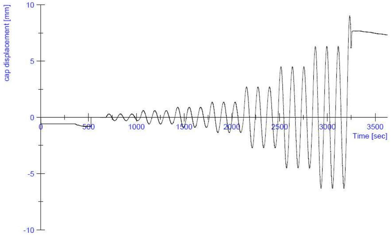
**Figure 38:** Progress of the horizontal displacement during the test on specimen CS02
