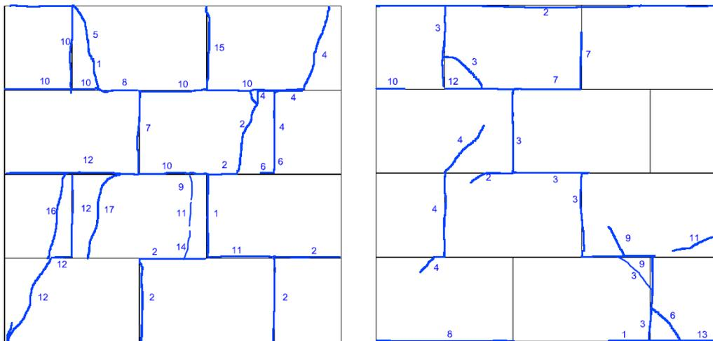
**Figure 12:** Crack pattern of the specimen CS03 and CS05
