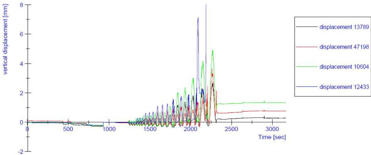
**Figure 75:** Progress of the vertical displacements during the test on specimen CS05
