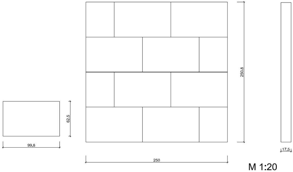
Figure 42: Dimension of the test specimen CS03
