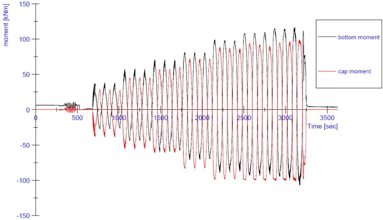
**Figure 40:** Progress of the in-plane bending moments at the top and at the bottom of the wall during the test on specimen CS02
