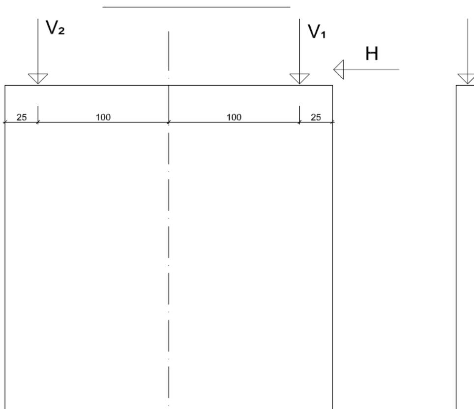
**Figure 91:** Position of the hydraulic actuators at test specimen CS07
