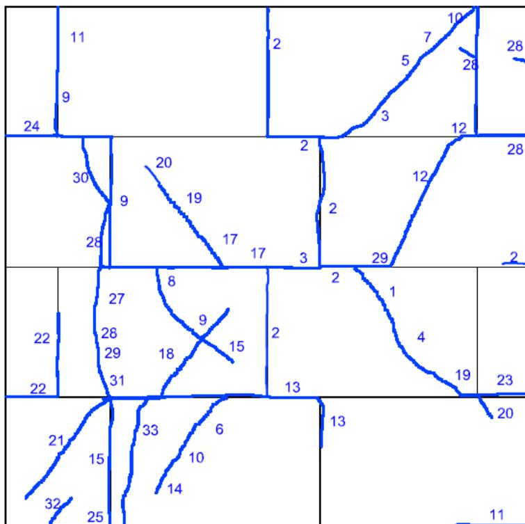
**Figure 81:** Crack pattern of the test specimen CS06
