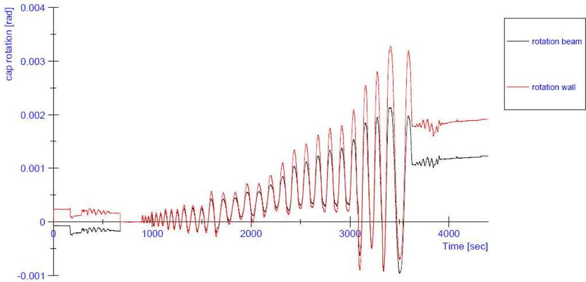
**Figure 53:** Progress of the in-plane rotation at the top of the wall during the test on specimen CS03
