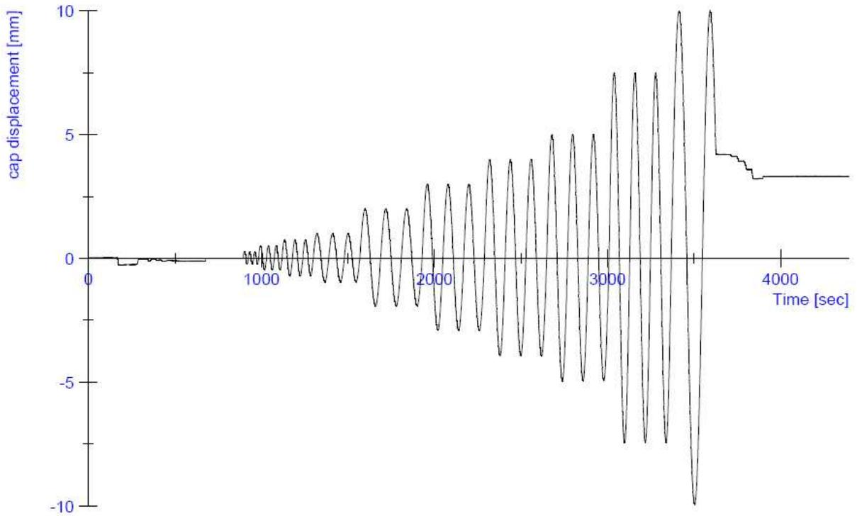
**Figure 50:** Progress of the horizontal displacement during the test on specimen CS03
