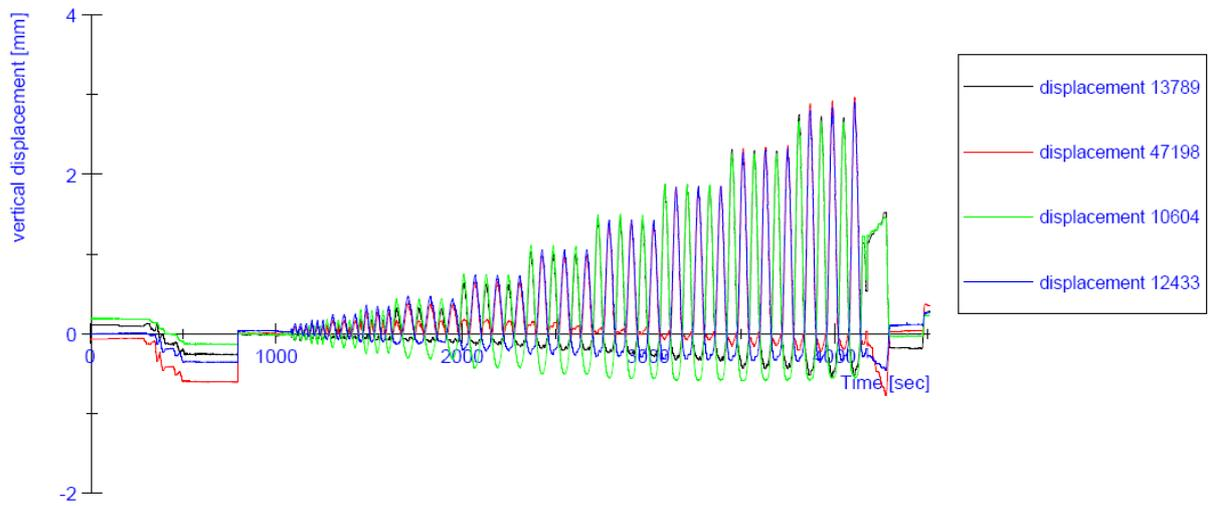
**Figure 63:** Progress of the vertical displacements during the test on specimen CS04
