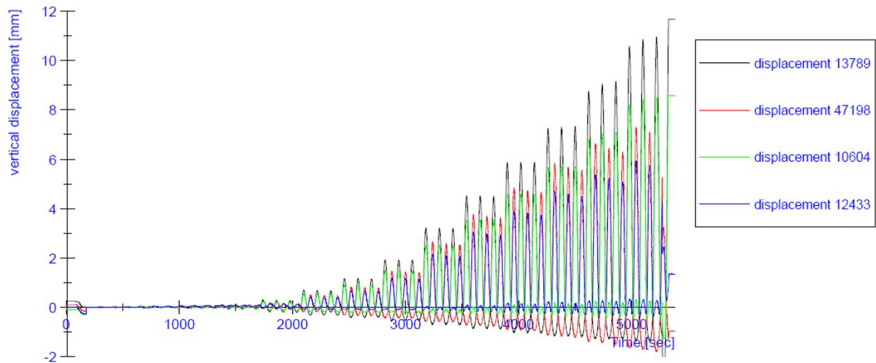
**Figure 111:** Progress of the vertical displacements during the test on specimen Clay01
