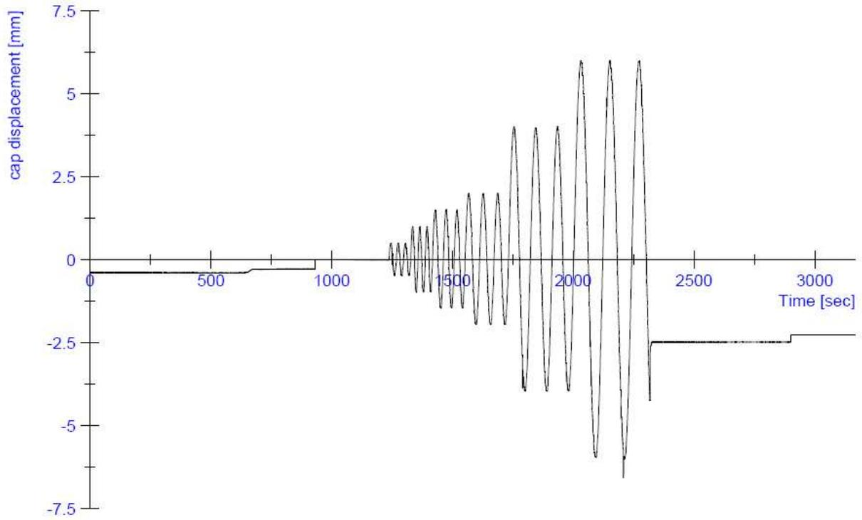
**Figure 74:** Progress of the horizontal displacement during the test on specimen CS05
