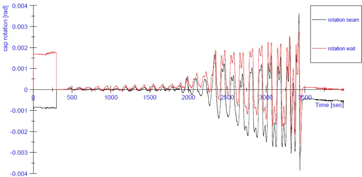
**Figure 29:** Progress of the in-plane rotation at the top of the wall during the test on specimen CS01
