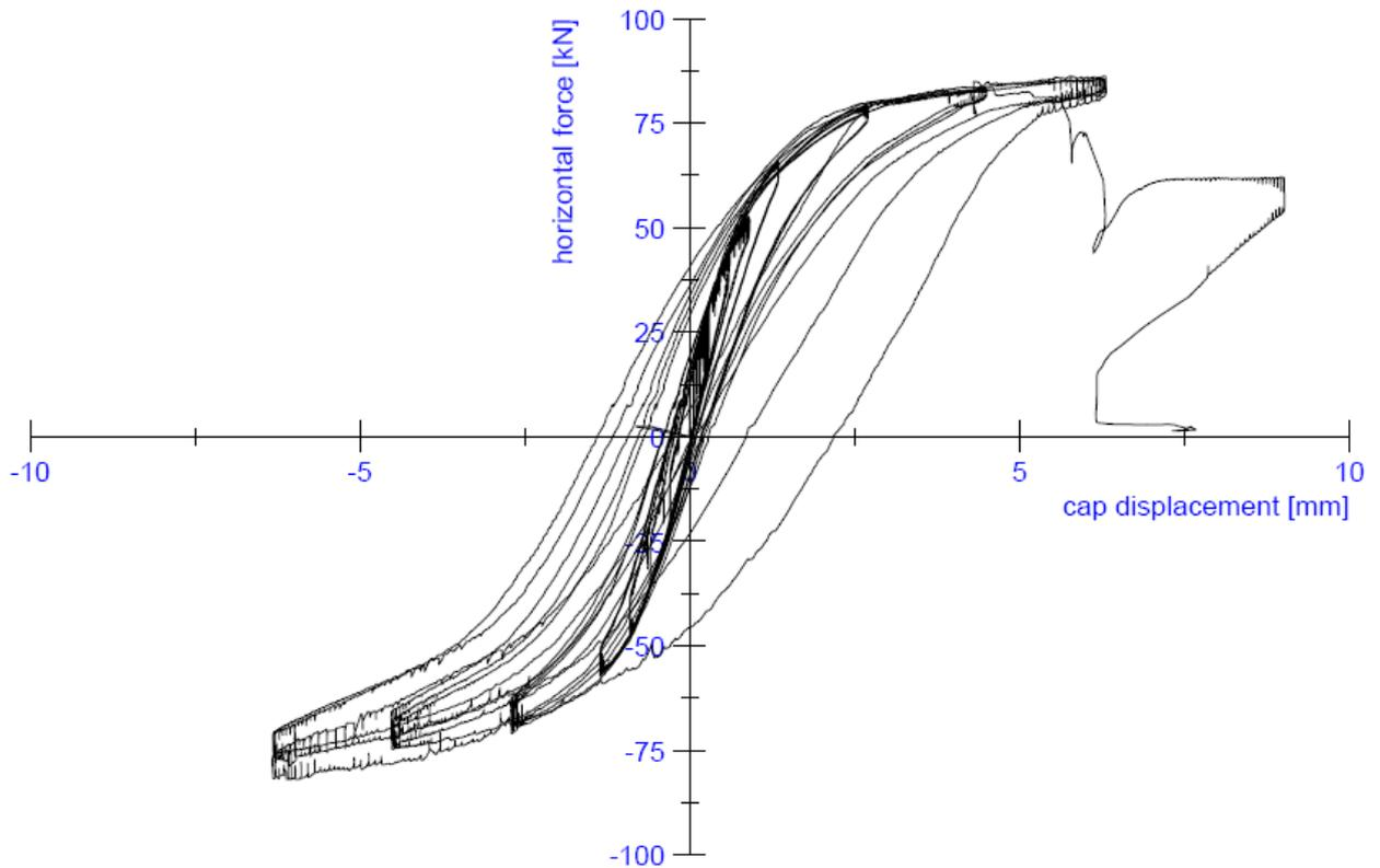
Figure 35: Load-displacement curve (hysteresis) of the test on specimen CS02
