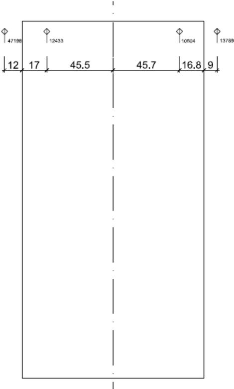
Figure 20: Position of the LVDTs at test specimen CS01
