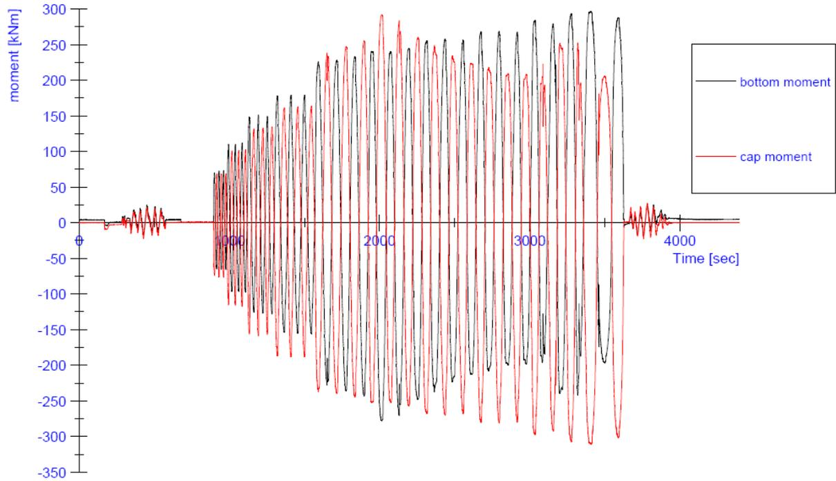
**Figure 52:** Progress of the in-plane bending moments at the top and at the bottom of the wall during the test on specimen CS03
