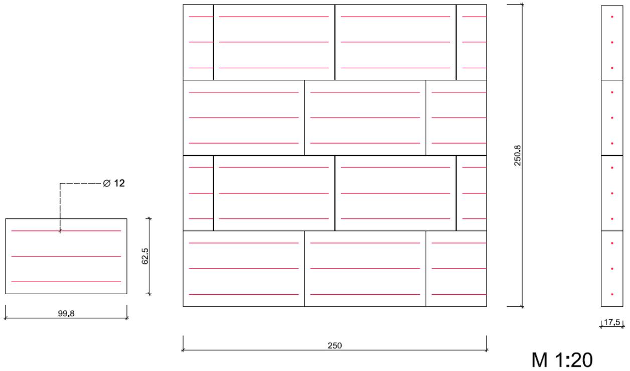
**Figure 78:** Dimension of the test specimen CS06 with the internal reinforcement
