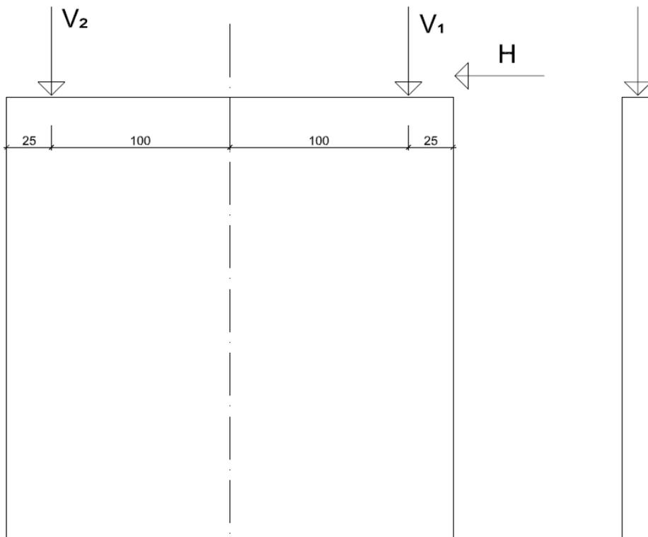
**Figure 79:** Position of the hydraulic actuators at test specimen CS06
