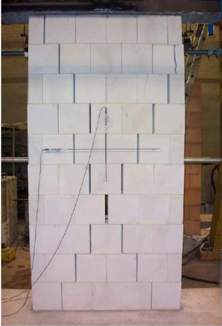
Figure 22: Crack pattern of the test specimen CS01
