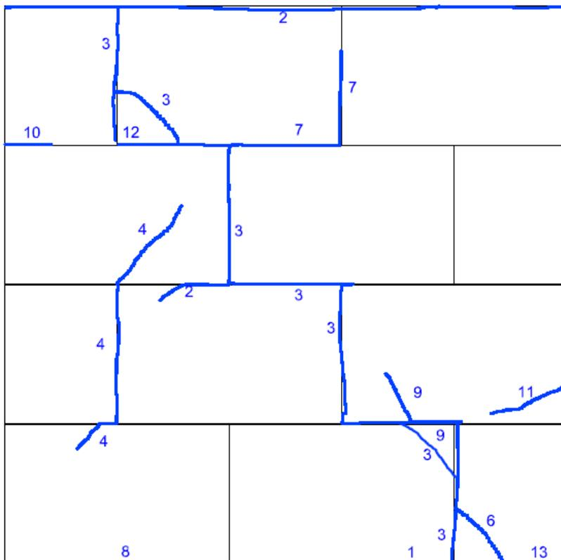
**Figure 69:** Crack pattern of the test specimen CS05
