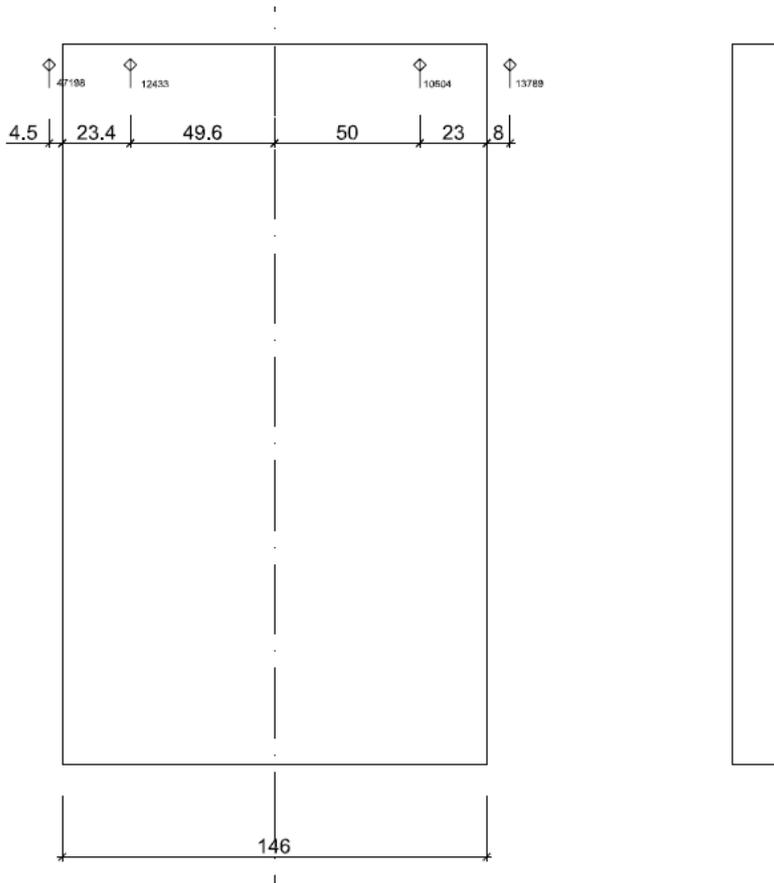
**Figure 104:** Position of the LVDTs at test specimen Clay01
