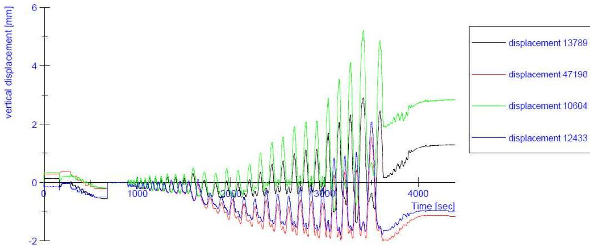
**Figure 51:** Progress of the vertical displacements during the test on specimen CS03
