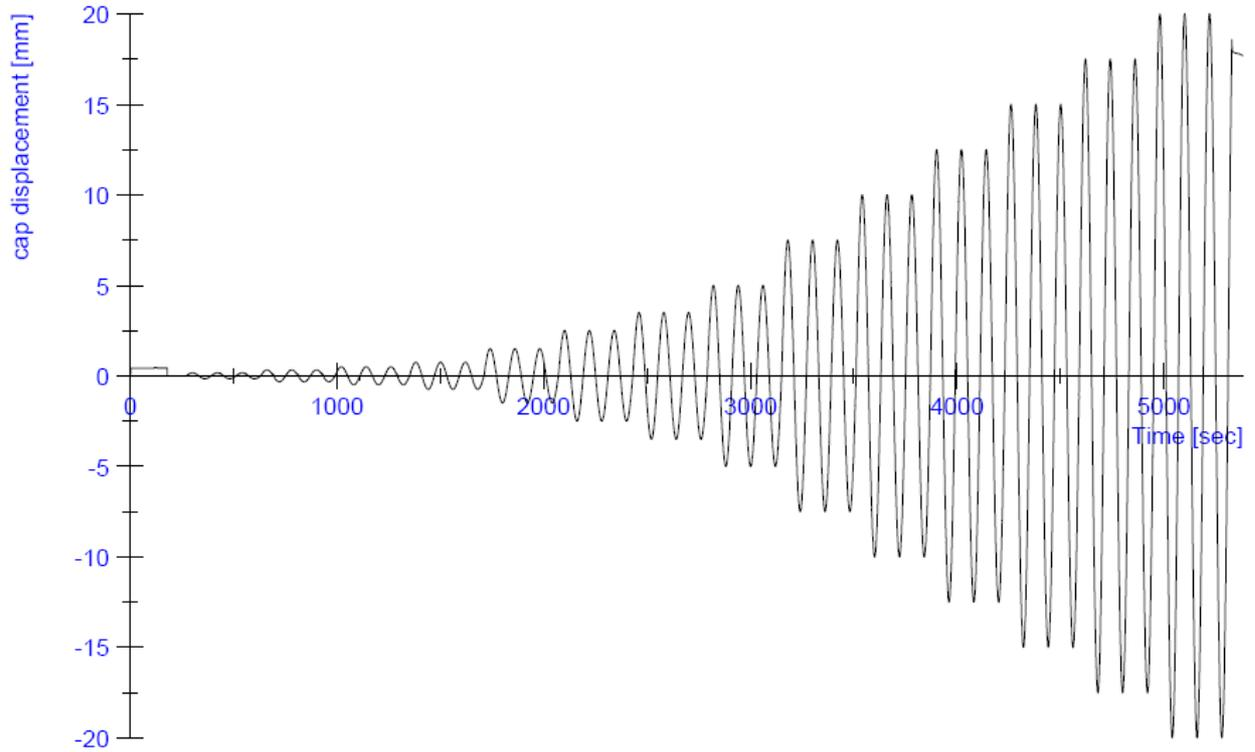
**Figure 110:** Progress of the horizontal displacement during the test on specimen Clay01
