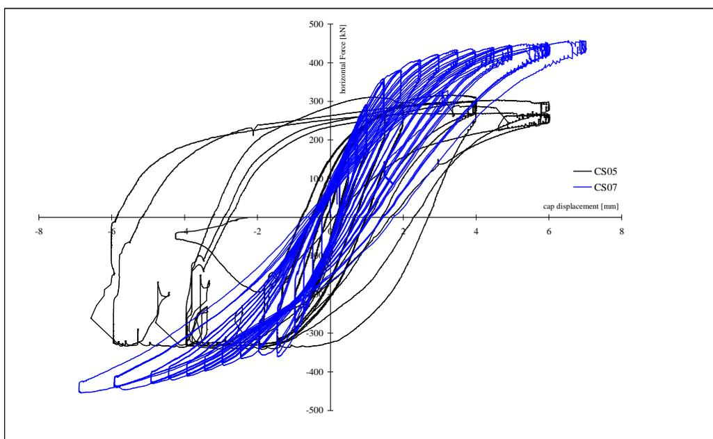
**Figure 9:** Hysteresis of the tests on the specimen CS05 and CS07
