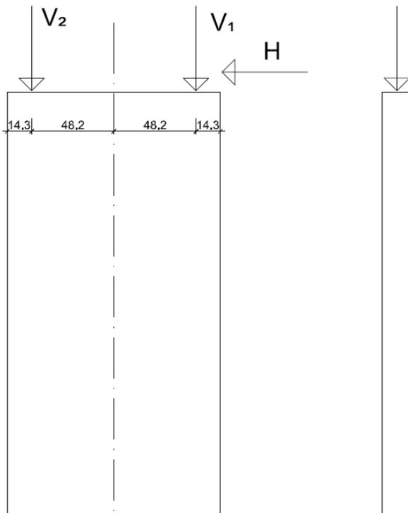
**Figure 19:** Position of the hydraulic actuators at test specimen CS01
