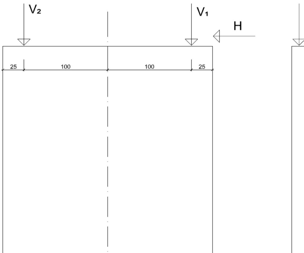
Figure 43: Position of the hydraulic actuators at test specimen CS03
