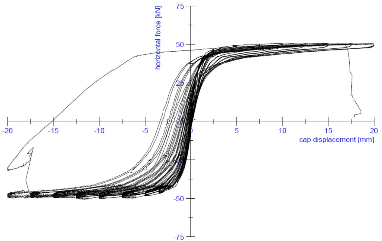
Figure 107: Load-displacement curve (hysteresis) of the test on specimen Clay01
