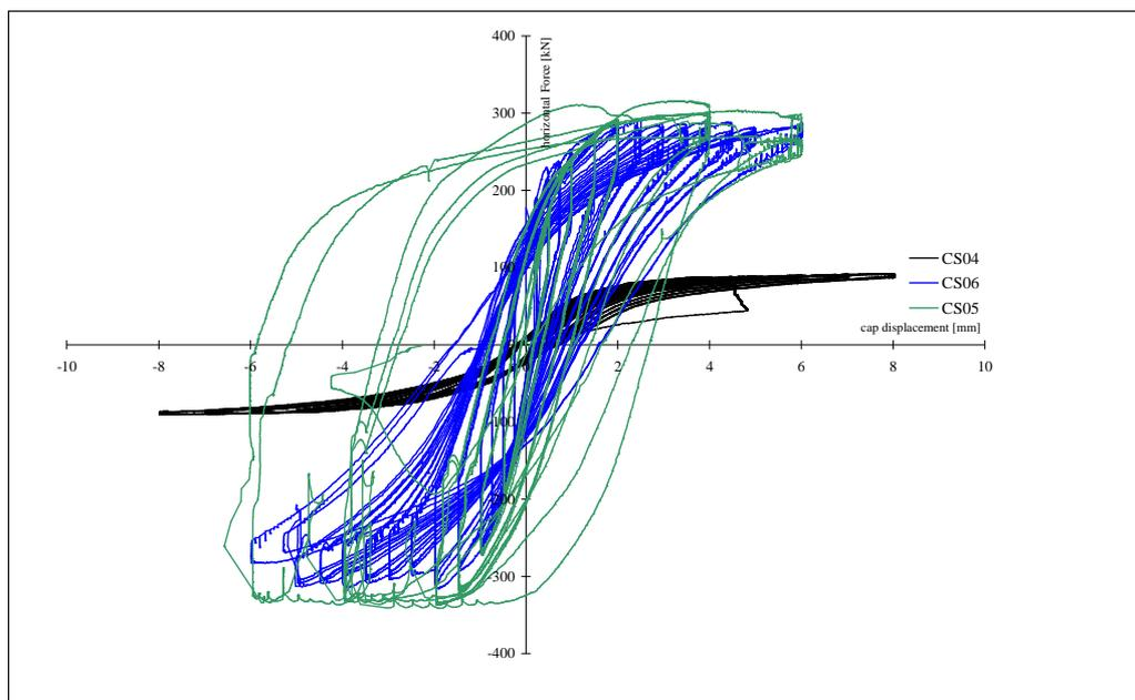
Figure 17: Hysteresis of the tests on the specimen CS04, CS05 and CS06
