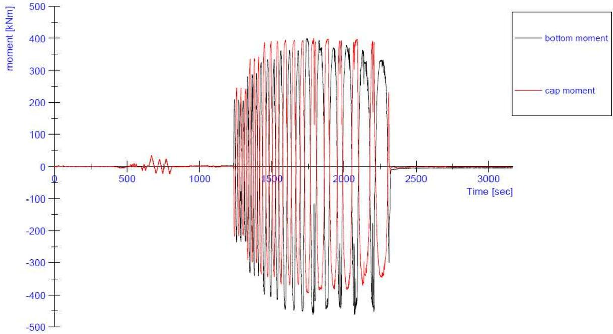
**Figure 76:** Progress of the in-plane bending moments at the top and at the bottom of the wall during the test on specimen CS05
