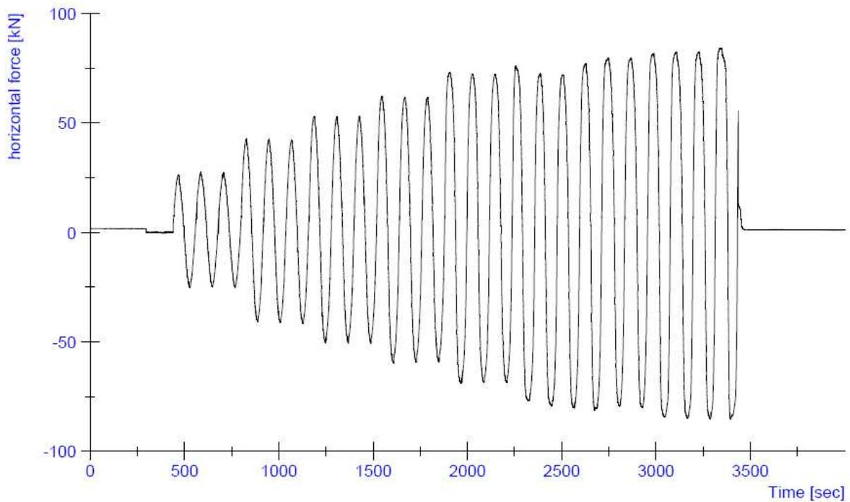
**Figure 25:** Progress of the horizontal force H during the test on specimen CS01
