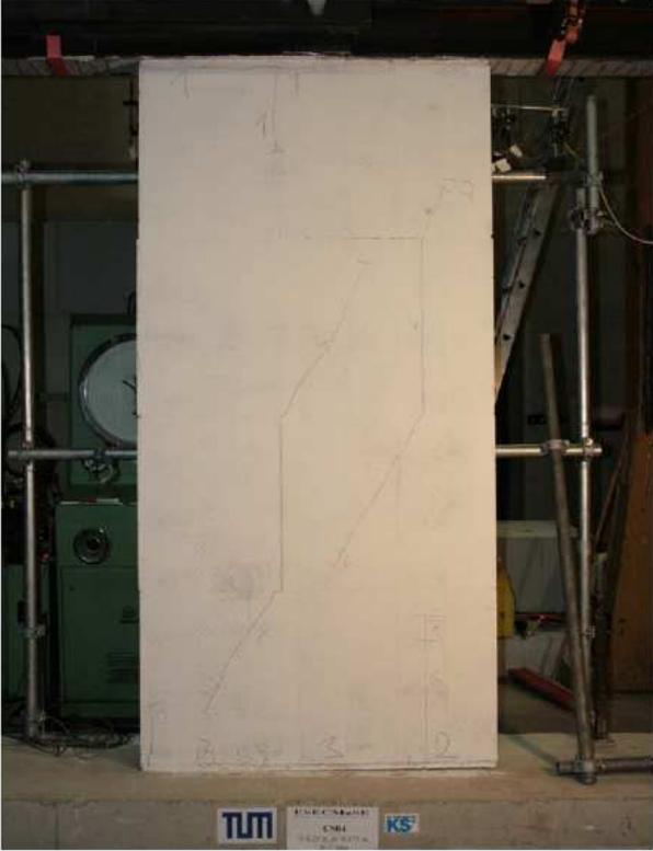
Figure 58: Crack pattern of the test specimen CS04
