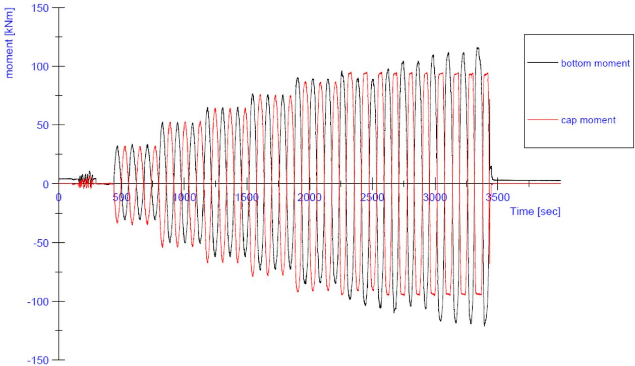
**Figure 28:** Progress of the in-plane bending moments at the top and at the bottom of the wall during the test on specimen CS01
