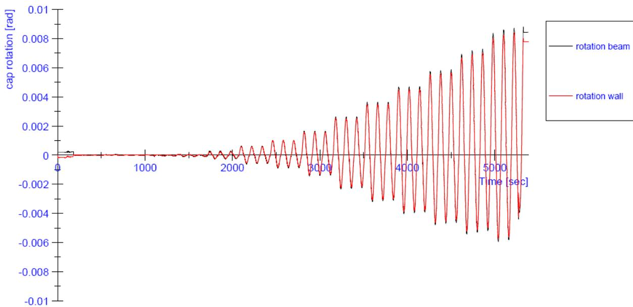
**Figure 113:** Progress of the in-plane rotation at the top of the wall during the test on specimen Clay01
