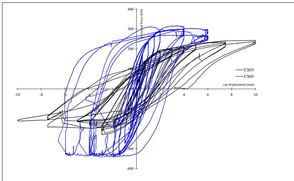
**Figure 13:** Hysteresis of the tests on the specimen CS03 and CS05
