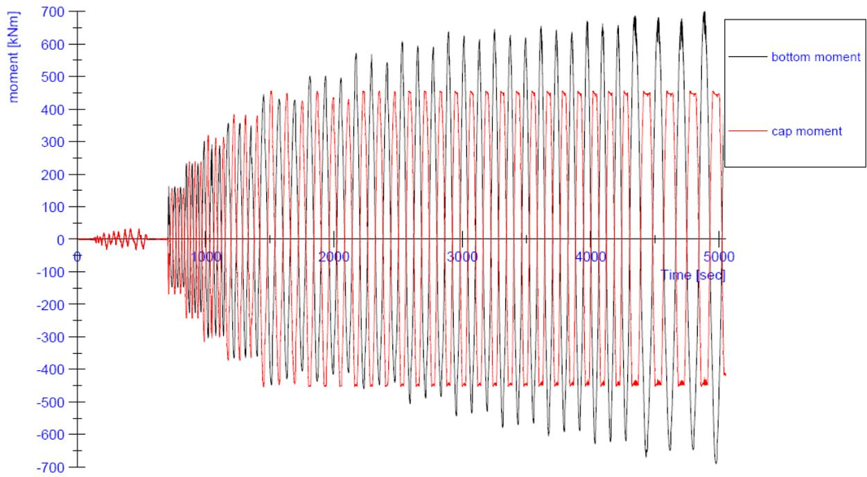
**Figure 100:** Progress of the in-plane bending moments at the top and at the bottom of the wall during the test on specimen CS07
