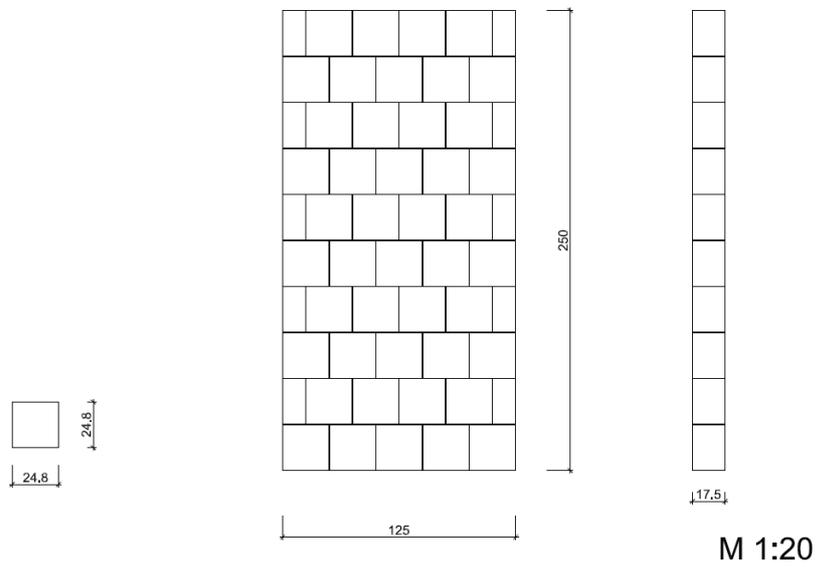
**Figure 18:** Dimension of the test specimen CS01
