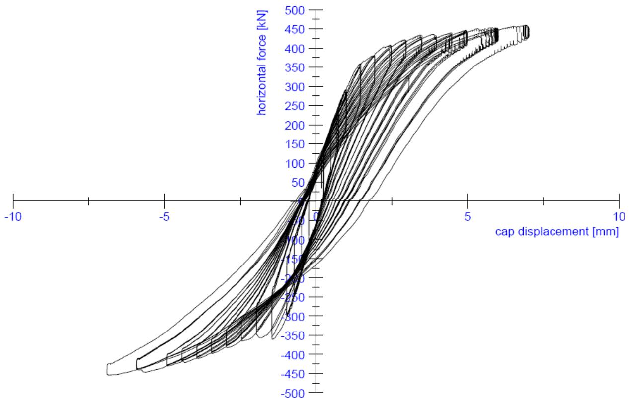
Figure 95: Load-displacement curve (hysteresis) of the test on specimen CS07
