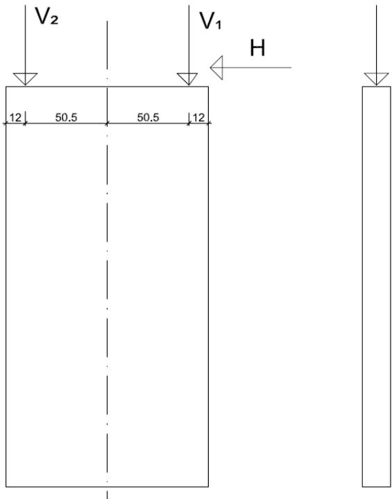
**Figure 31:** Position of the hydraulic actuators at test specimen CS02
