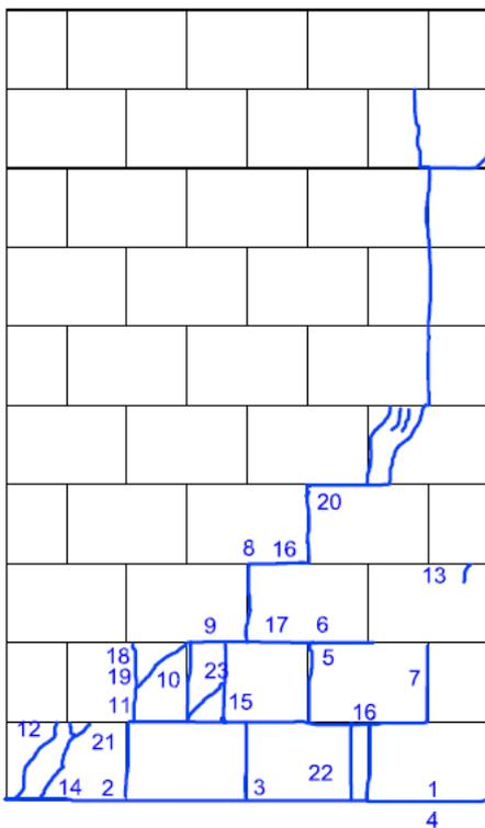
**Figure 105:** Crack pattern of the test specimen Clay01
