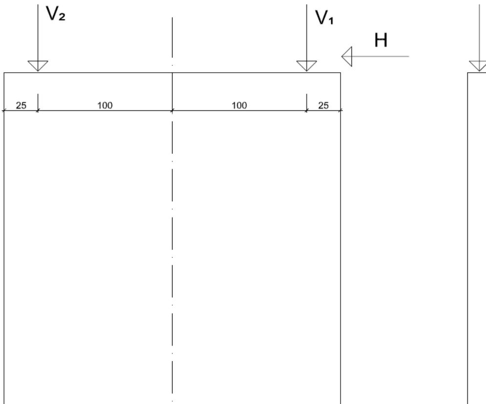
**Figure 67:** Position of the hydraulic actuators at test specimen CS05
