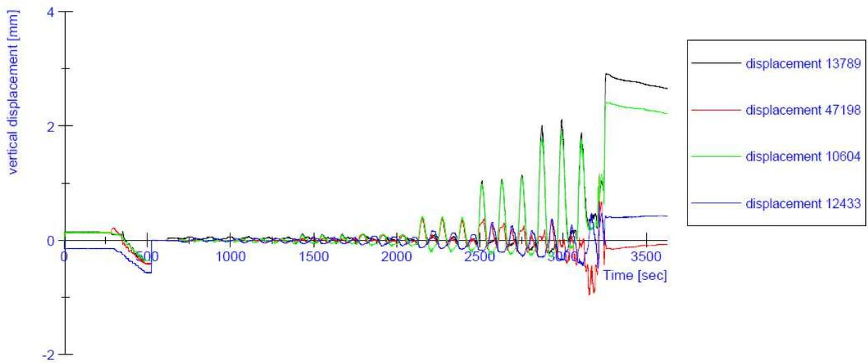
**Figure 39:** Progress of the vertical displacements during the test on specimen CS02
