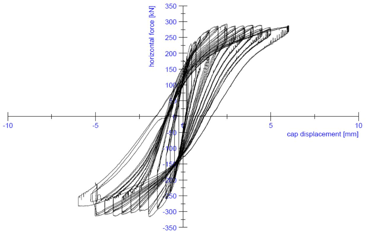
Figure 83: Load-displacement curve (hysteresis) of the test on specimen CS06
