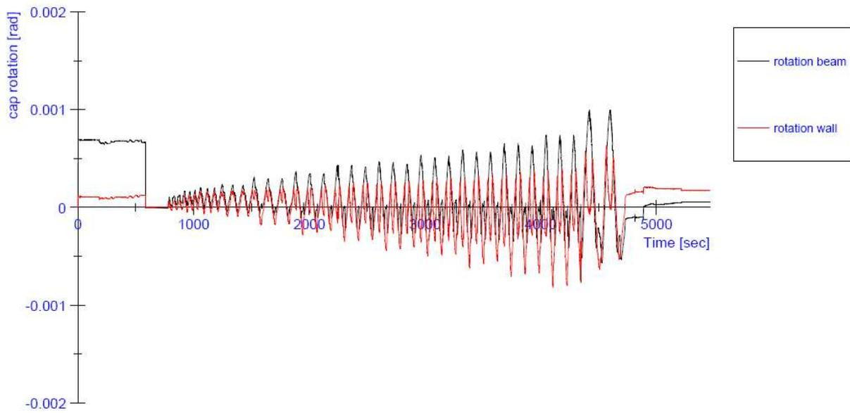
**Figure 89:** Progress of the in-plane rotation at the top of the wall during the test on specimen CS06
