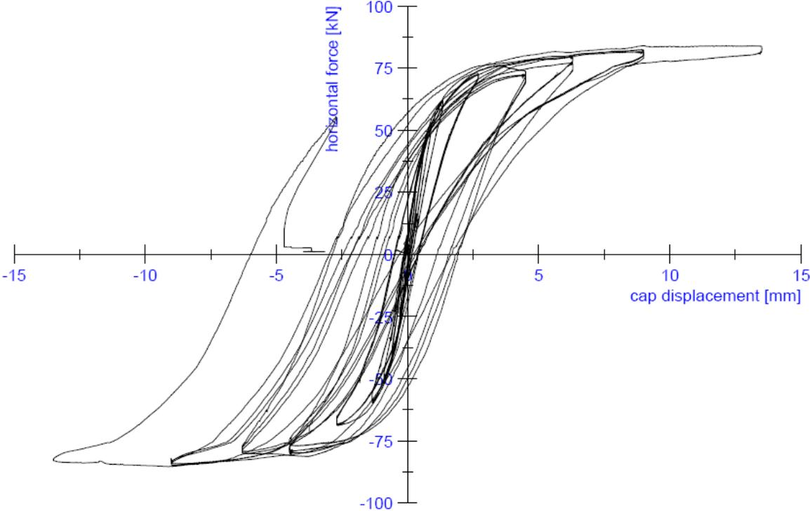
Figure 23: Load-displacement curve (hysteresis) of the test on specimen CS01
