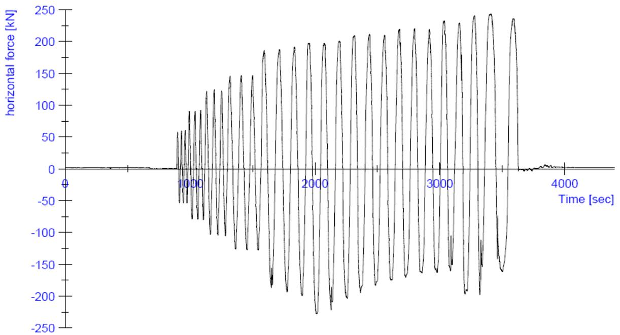
**Figure 49:** Progress of the horizontal force H during the test on specimen CS03
