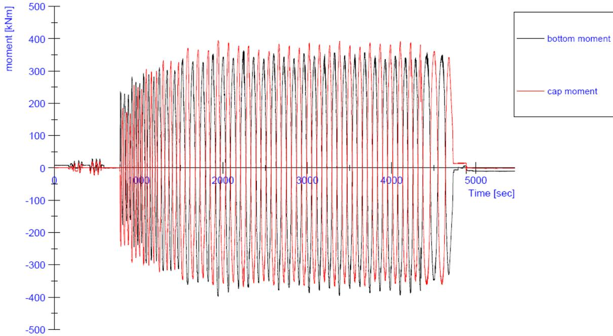
**Figure 88:** Progress of the in-plane bending moments at the top and at the bottom of the wall during the test on specimen CS06
