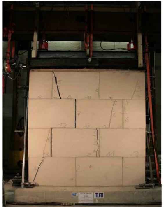
Figure 46: Crack pattern of the test specimen CS03
