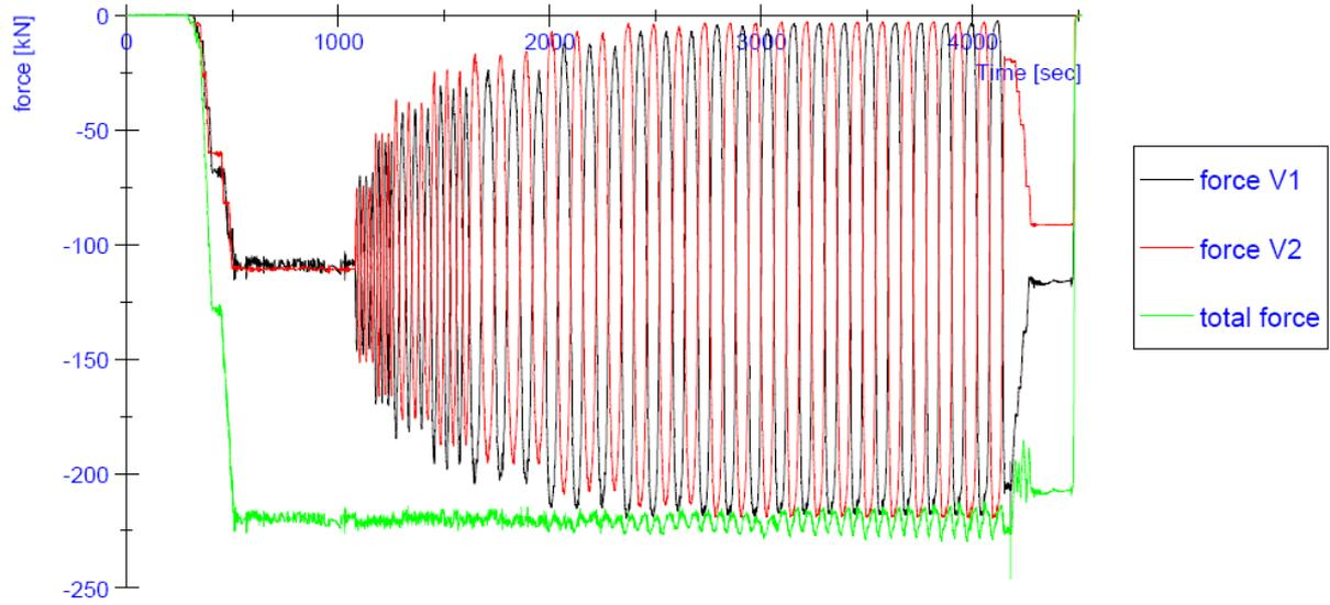
**Figure 60:** Progress of the vertical forces V1 and V2 during the test on specimen CS04
