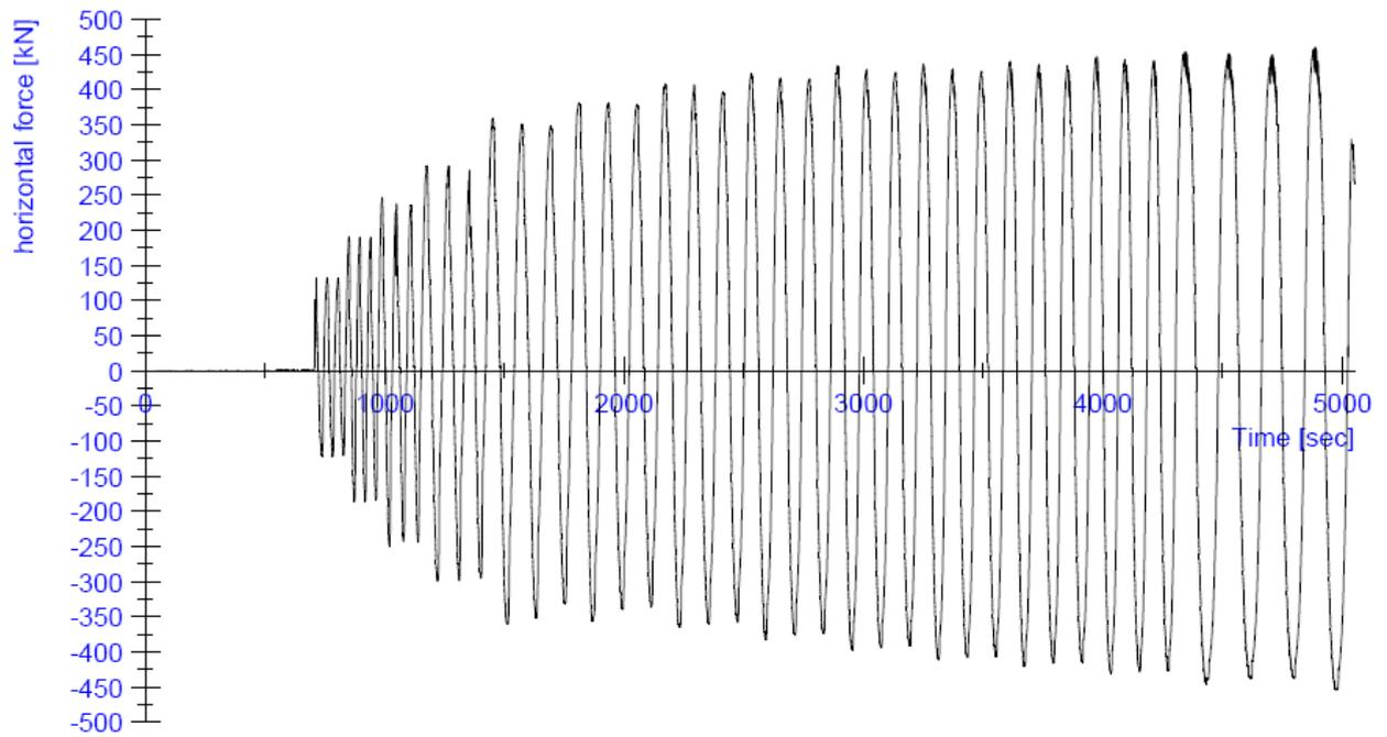
**Figure 97:** Progress of the horizontal force H during the test on specimen CS07
