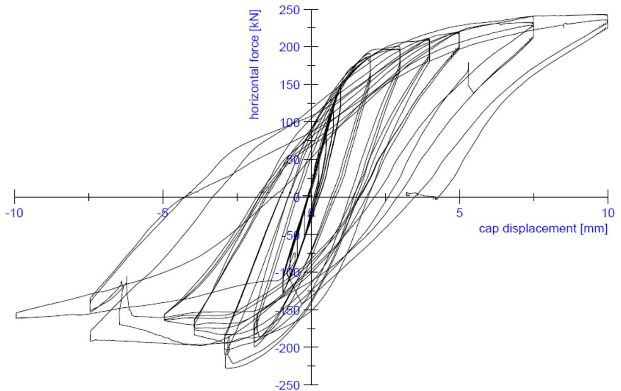
Figure 47: Load-displacement curve (hysteresis) of the test on specimen CS03
