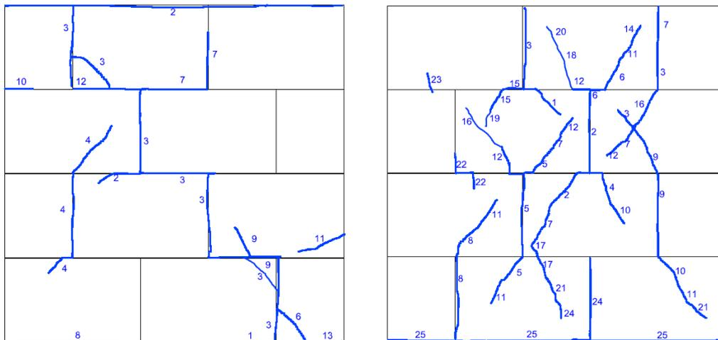
**Figure 8:** Crack pattern of the specimen CS05 and CS07
