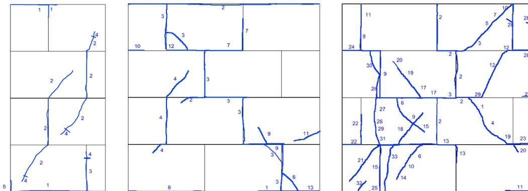
Figure 16: Crack pattern of the specimen CS04, CS05 and CS06
