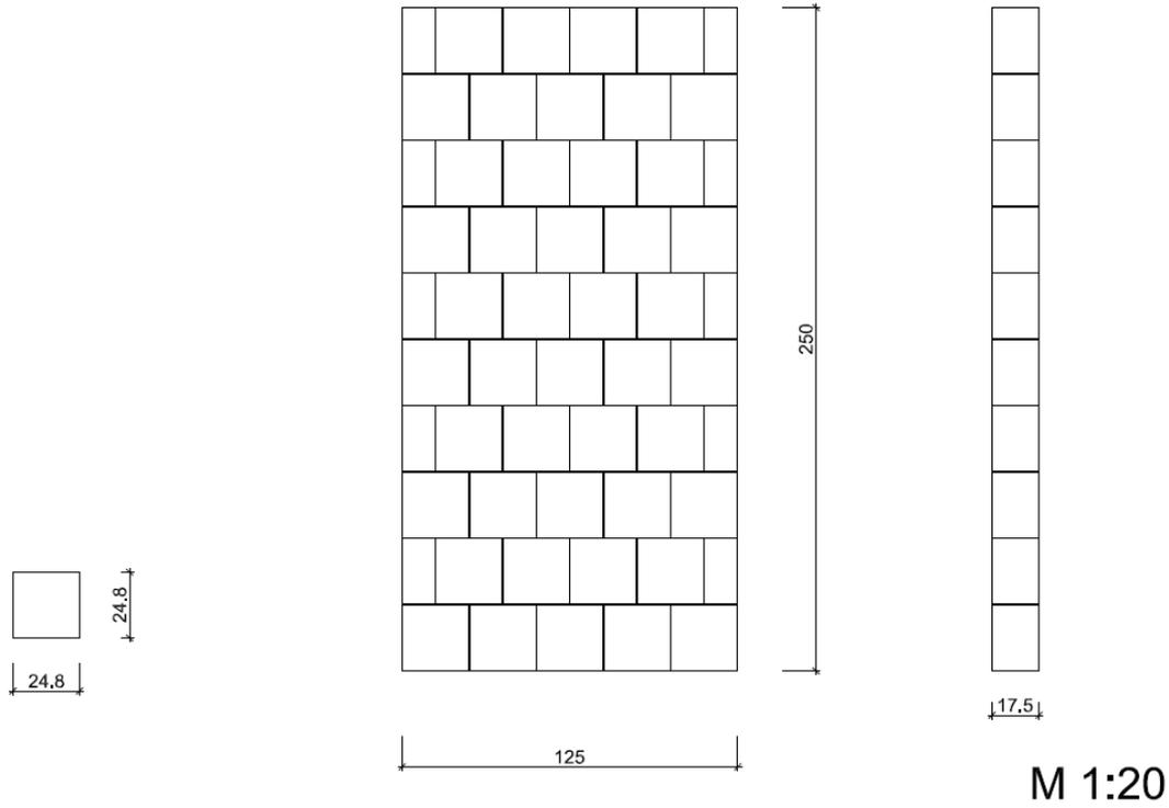
**Figure 30:** Dimension of the test specimen CS02
