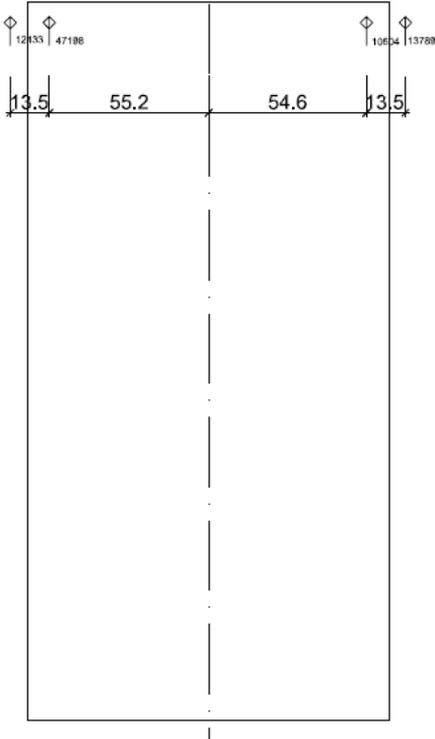
Figure 56: Position of the LVDTs at test specimen CS04
