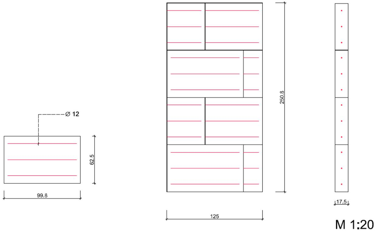
**Figure 54:** Dimension of the test specimen CS04 with the internal reinforcement
