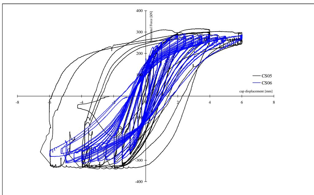
**Figure 15:** Hysteresis of the tests on the specimen CS05 and CS06
