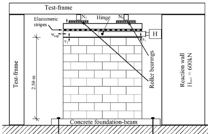
**Figure 7:** Test set-up used for the static-cyclic tests at the TU Munich [Deliverable 6]
