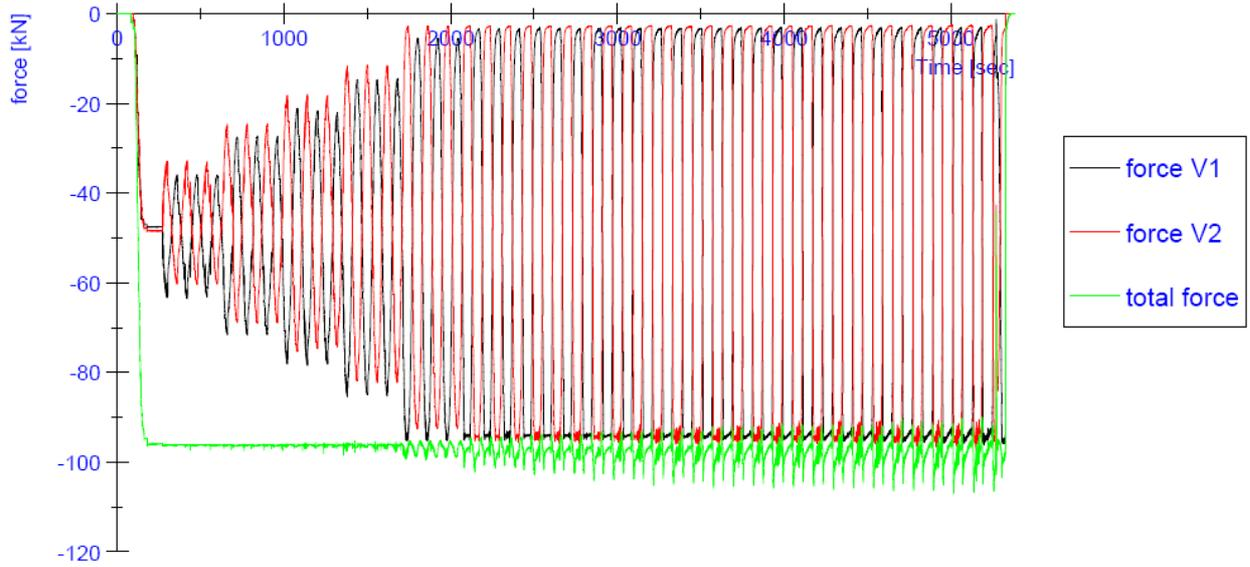
**Figure 108:** Progress of the vertical forces V1 and V2 during the test on specimen Clay01
