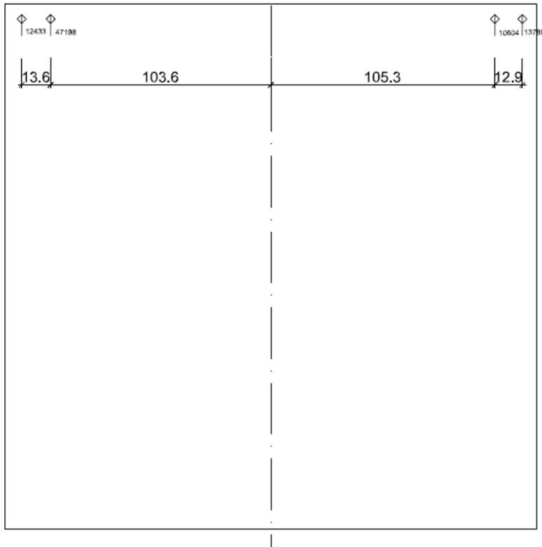
Figure 44: Position of the LVDTs at test specimen CS03
