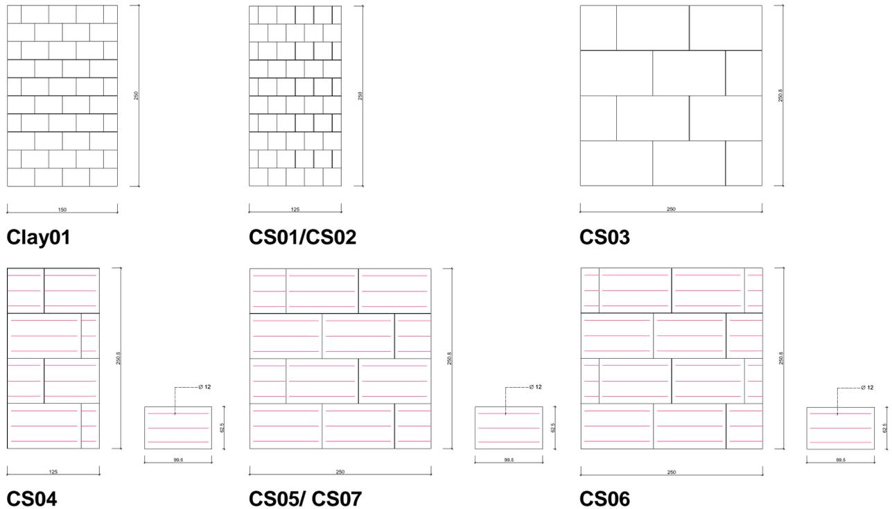
**Figure 1:** Overview of the wall specimen
