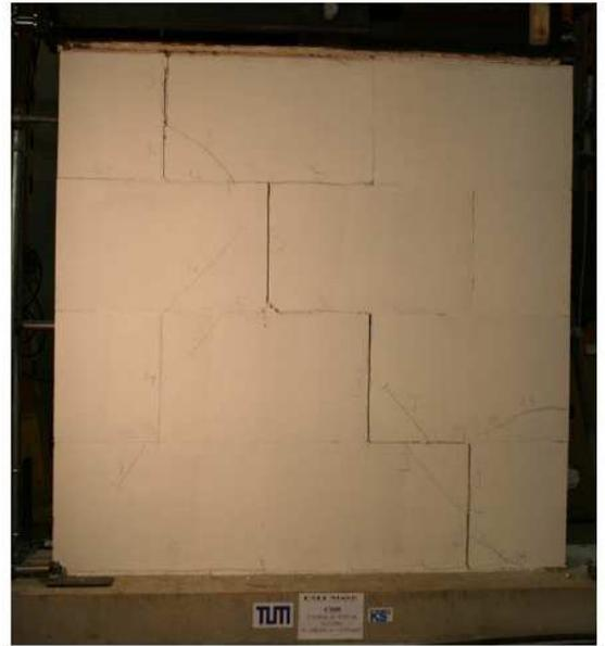
**Figure 70:** Crack pattern of the test specimen CS05
