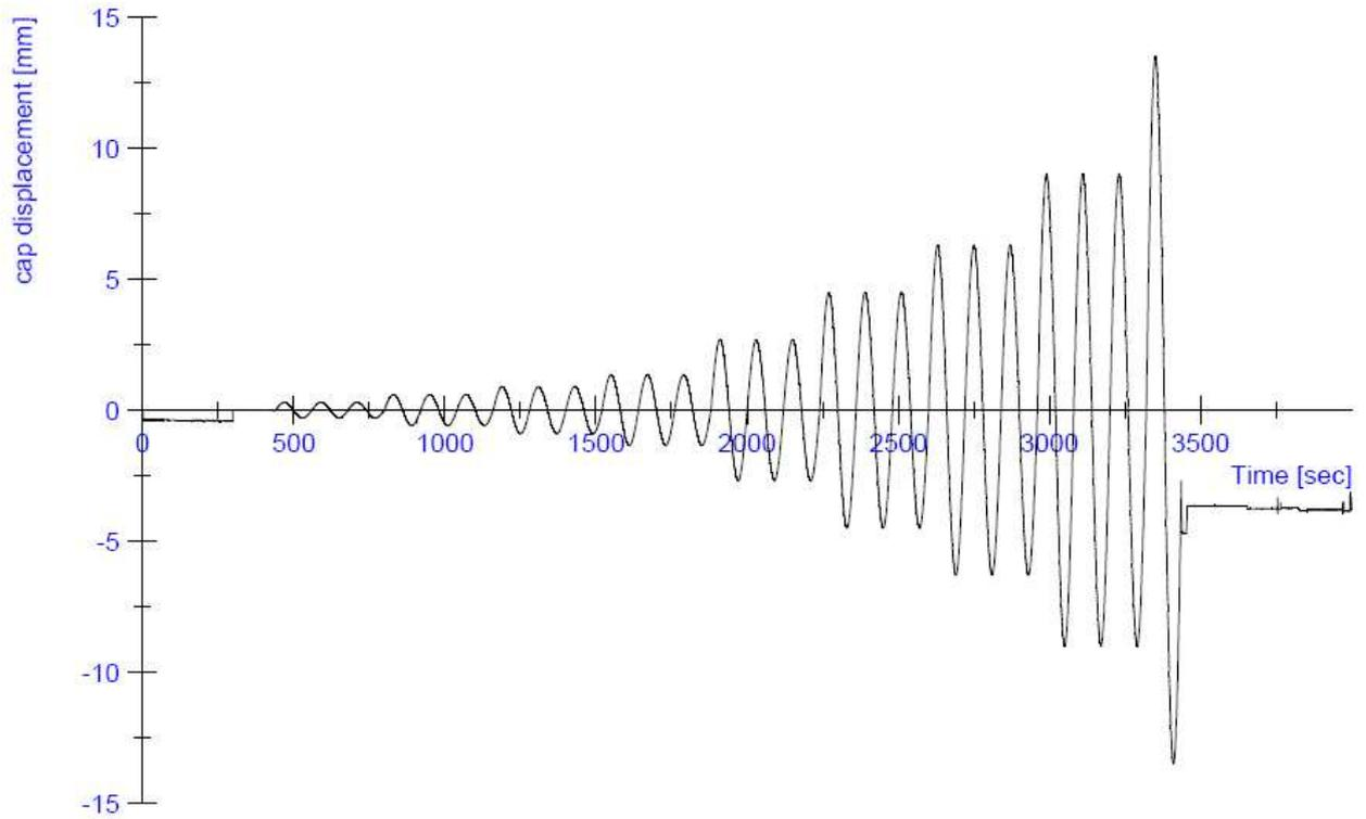
**Figure 26:** Progress of the horizontal displacement during the test on specimen CS01
