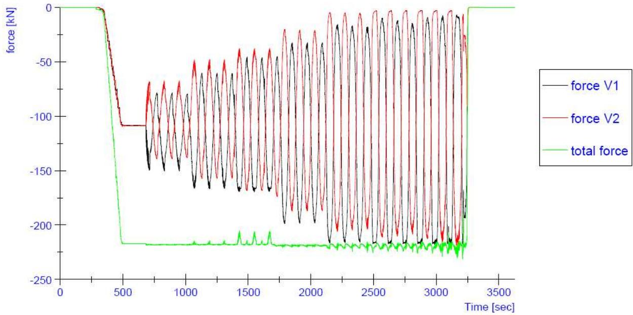
**Figure 36:** Progress of the vertical forces V1 and V2 during the test on specimen CS02
