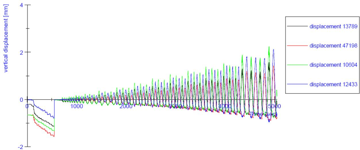
**Figure 99:** Progress of the vertical displacements during the test on specimen CS07
