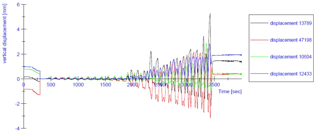
**Figure 27:** Progress of the vertical displacements during the test on specimen CS01
