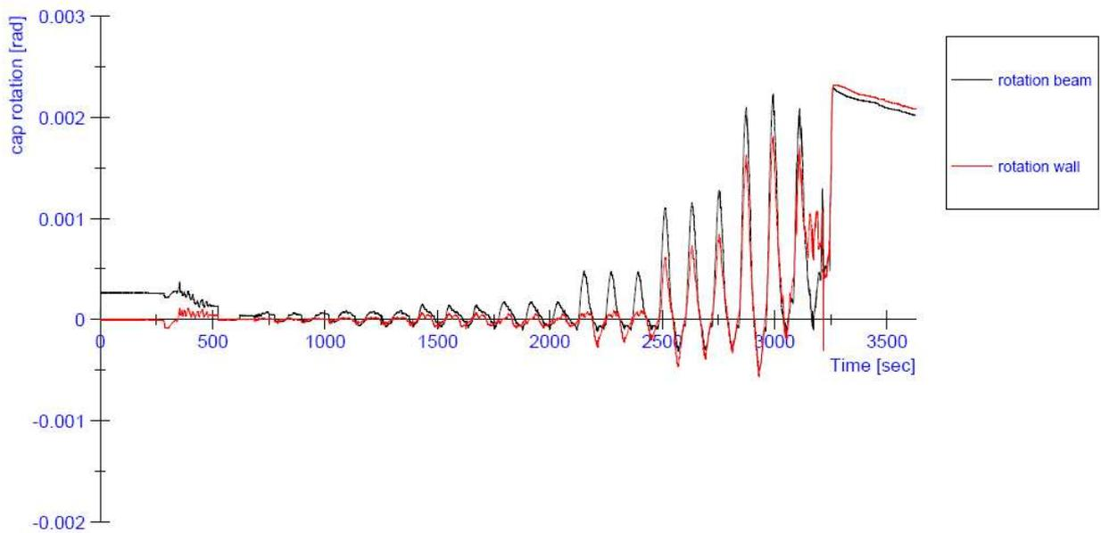
**Figure 41:** Progress of the in-plane rotation at the top of the wall during the test on specimen CS02
