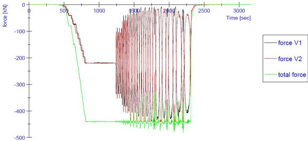
**Figure 72:** Progress of the vertical forces V1 and V2 during the test on specimen CS05
