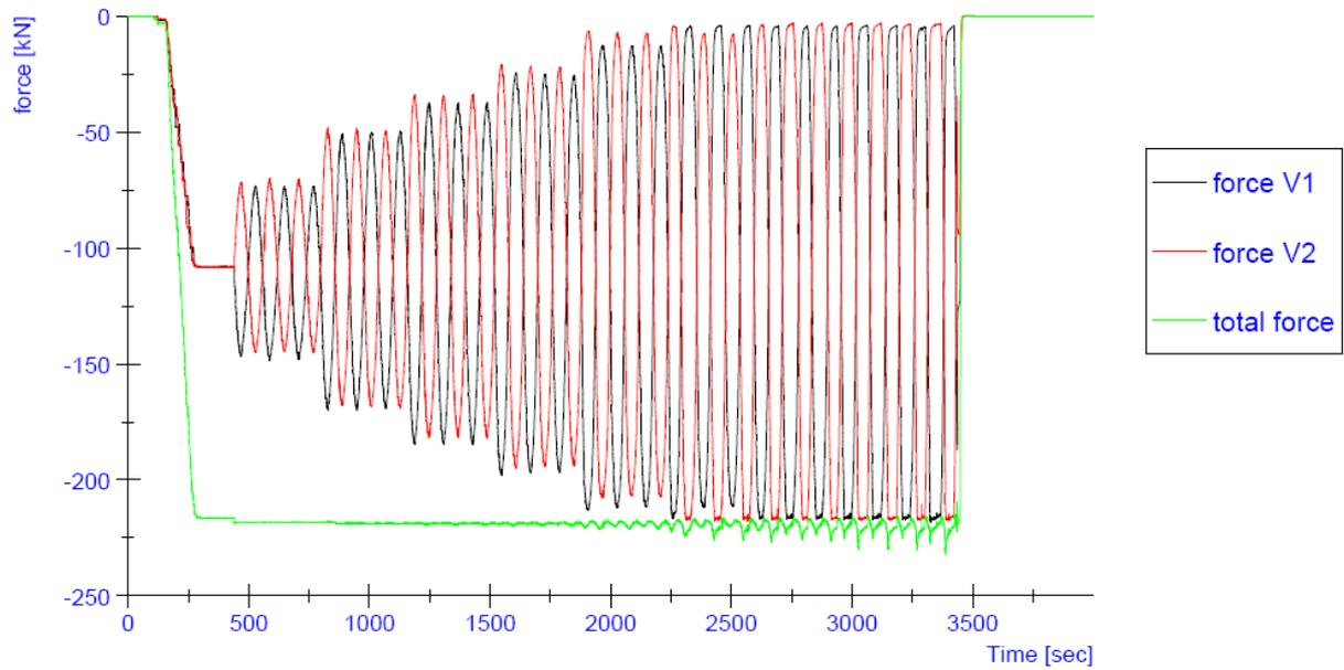
**Figure 24:** Progress of the vertical forces V1 and V2 during the test on specimen CS01
