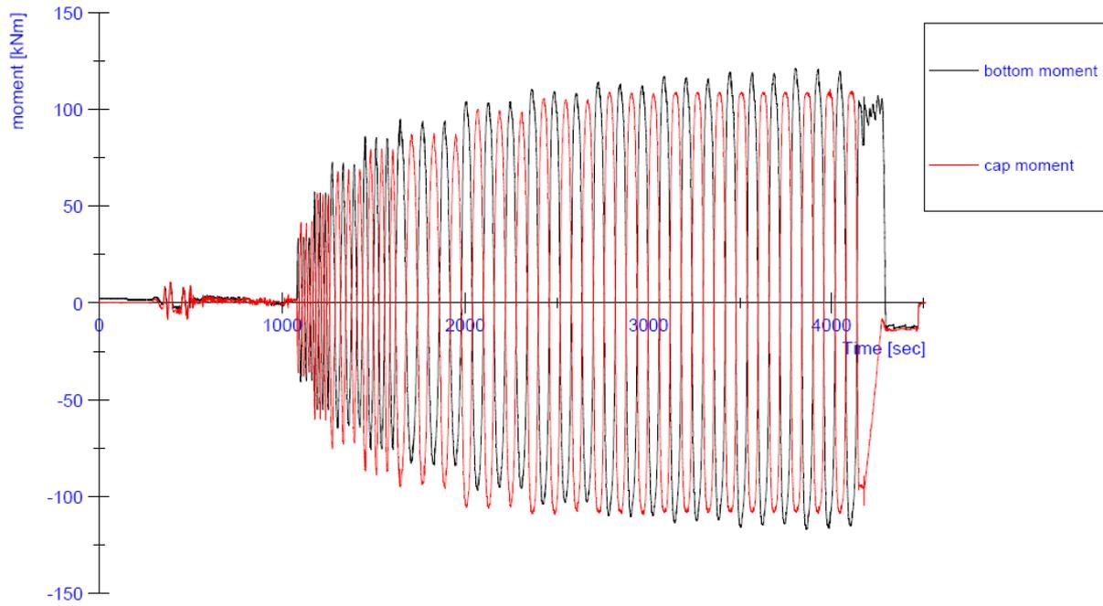
**Figure 64:** Progress of the in-plane bending moments at the top and at the bottom of the wall during the test on specimen CS04
