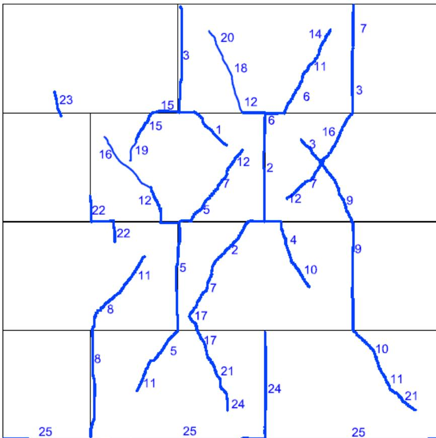
**Figure 93:** Crack pattern of the test specimen CS07
