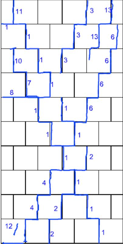
Figure 21: Crack pattern of the test specimen CS01
