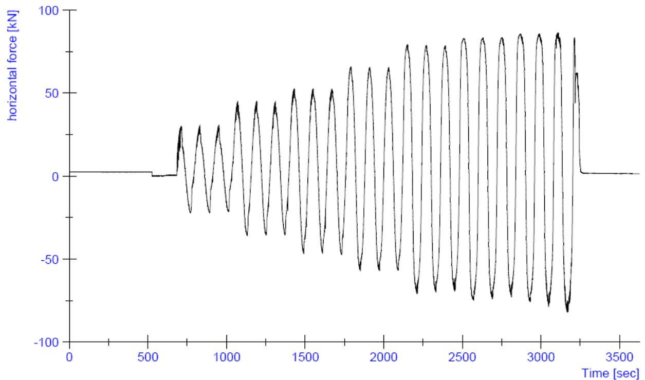
**Figure 37:** Progress of the horizontal force H during the test on specimen CS02
