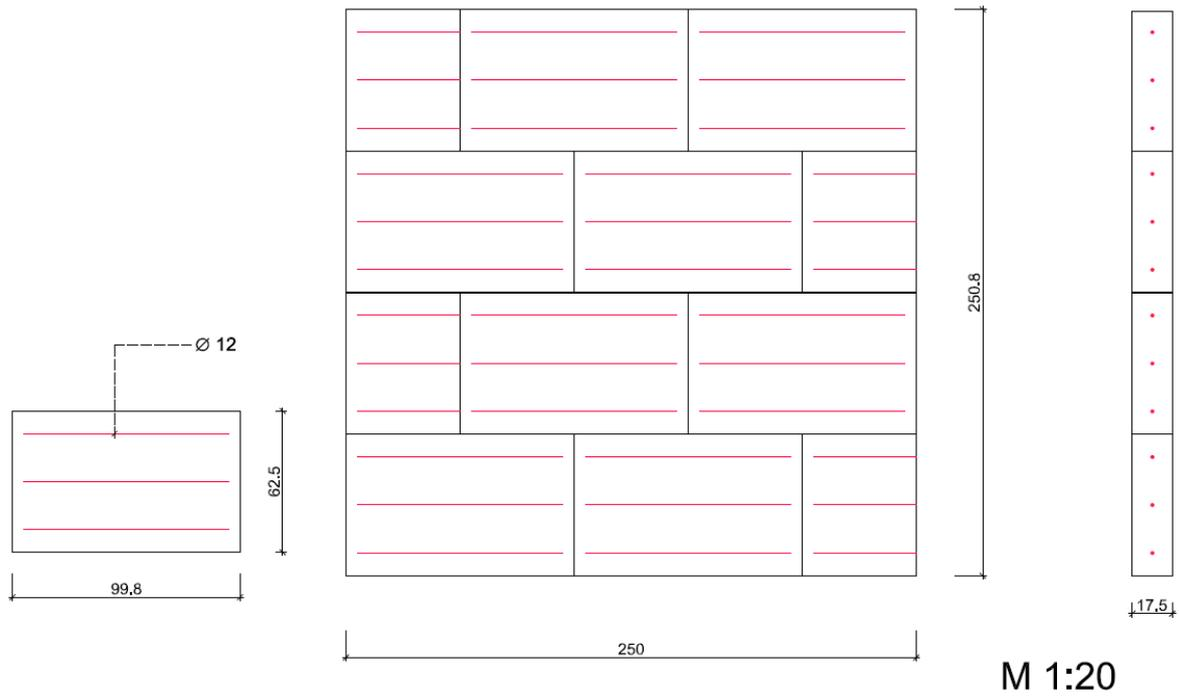
**Figure 90:** Dimension of the test specimen CS07 with the internal reinforcement
