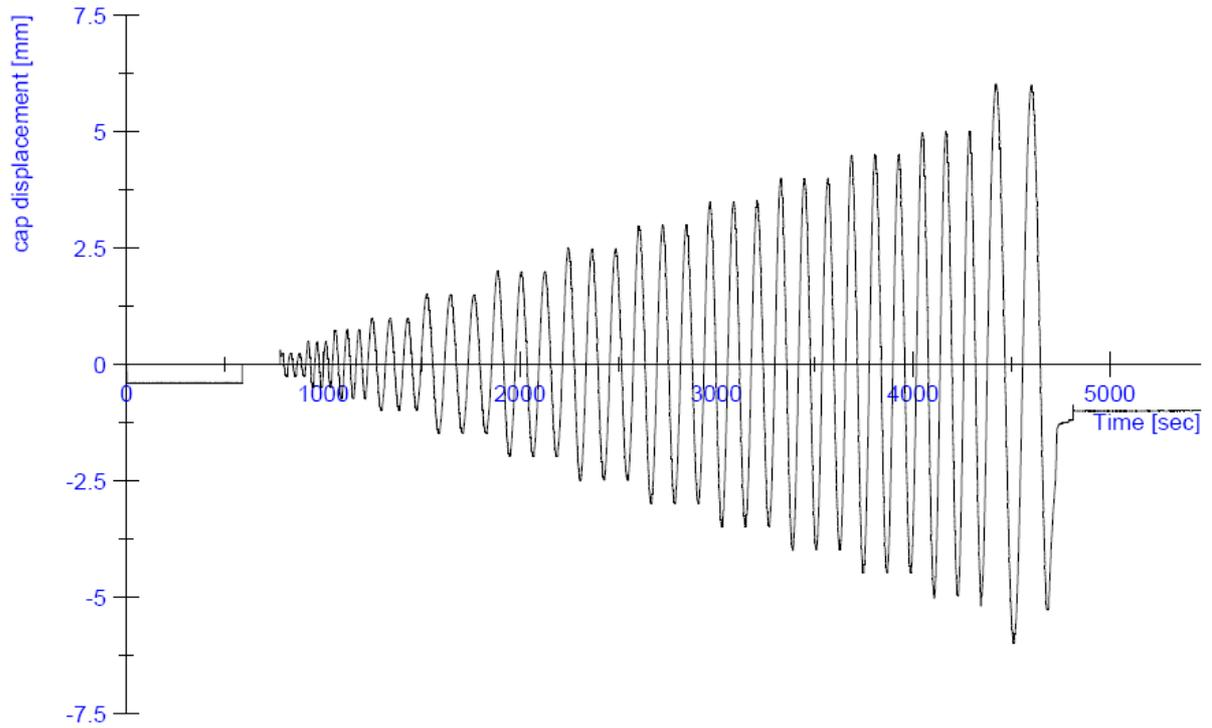
**Figure 86:** Progress of the horizontal displacement during the test on specimen CS06
