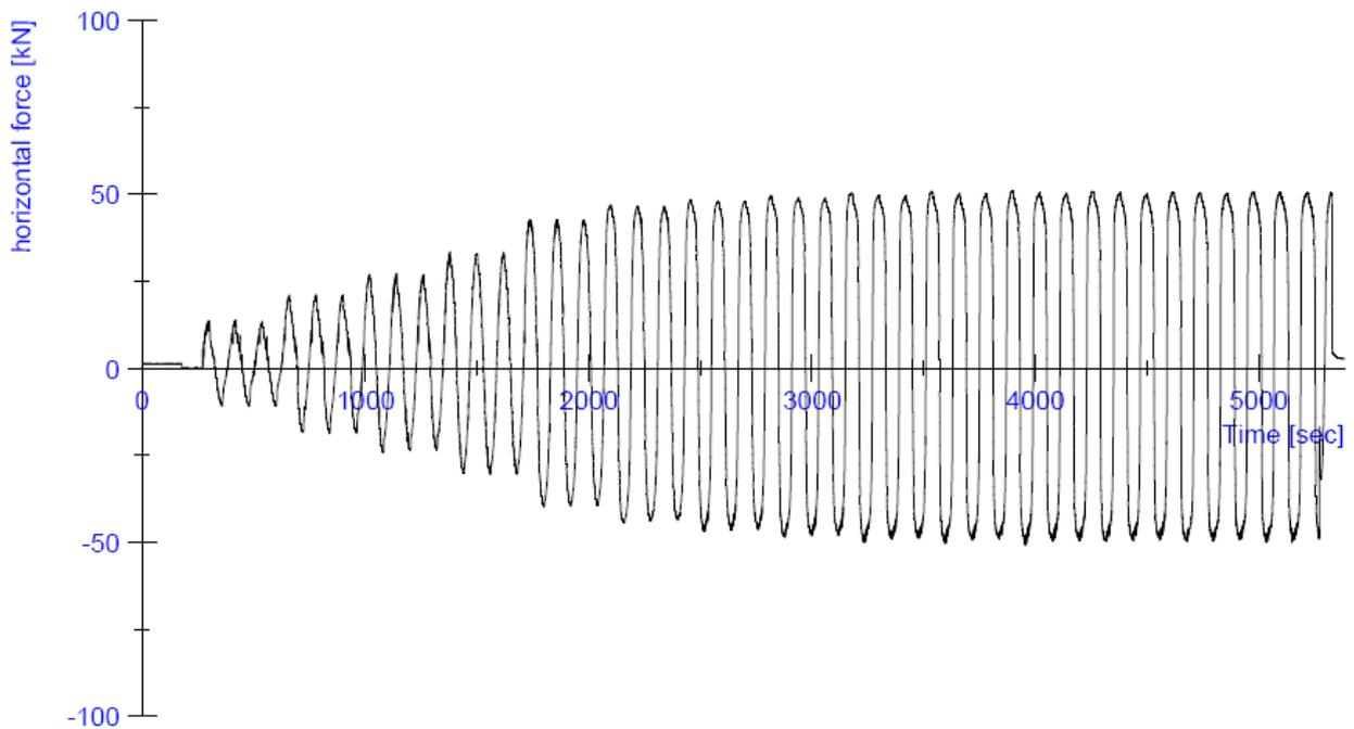
**Figure 109:** Progress of the horizontal force H during the test on specimen Clay01
