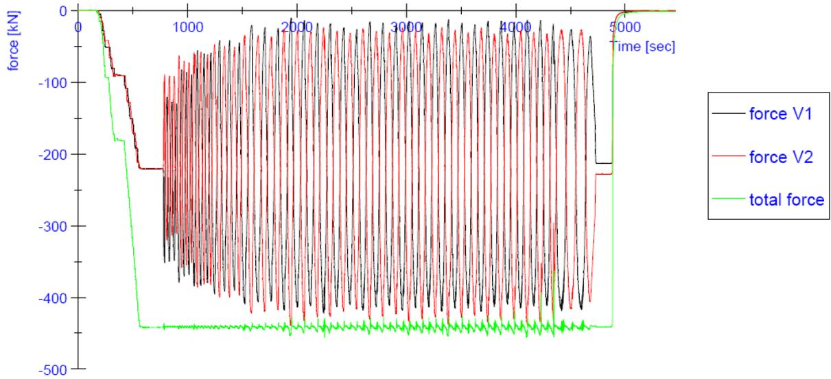
**Figure 84:** Progress of the vertical forces V1 and V2 during the test on specimen CS06
