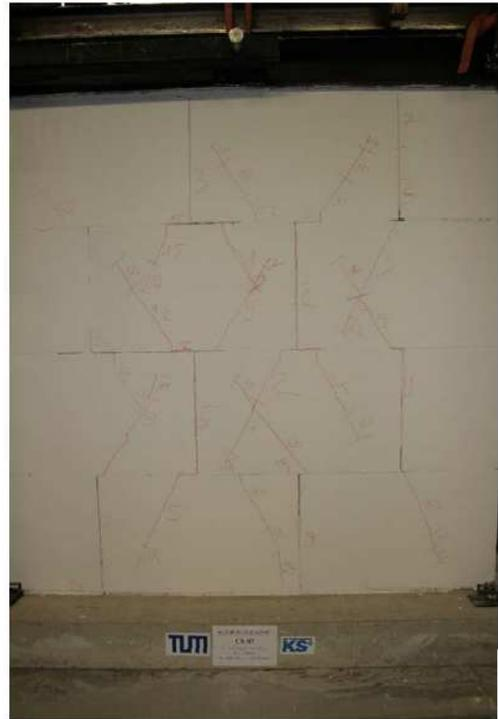
Figure 94: Crack pattern of the test specimen CS07
