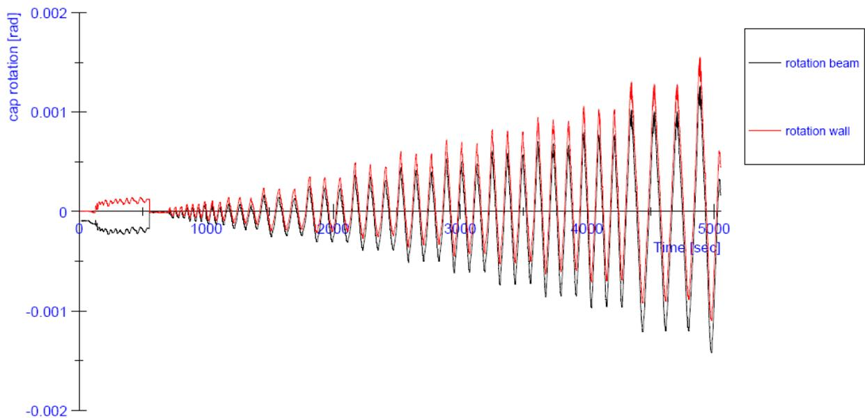
**Figure 101:** Progress of the in-plane rotation at the top of the wall during the test on specimen CS07
