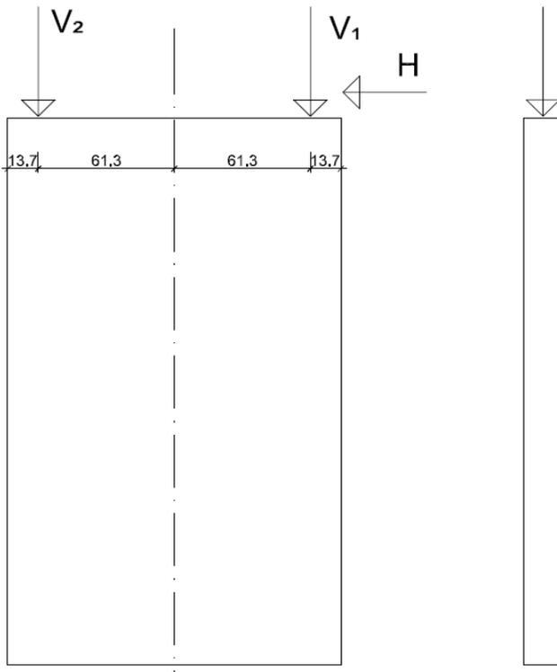
**Figure 103:** Position of the hydraulic actuators at test specimen Clay01
