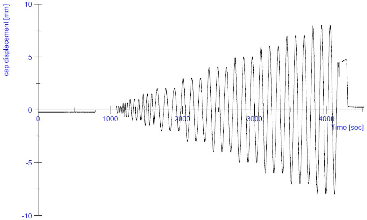
**Figure 62:** Progress of the horizontal displacement during the test on specimen CS04
