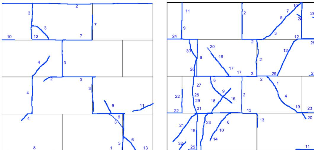
**Figure 14:** Crack pattern of the specimen CS05 and CS06
