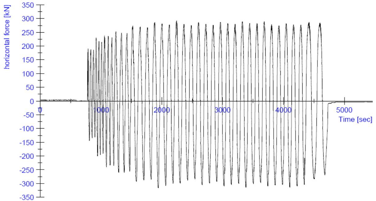
**Figure 85:** Progress of the horizontal force H during the test on specimen CS06
