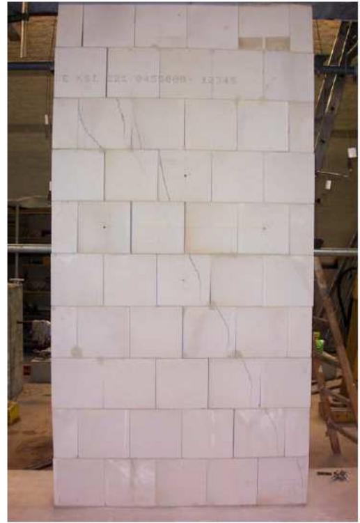
Figure 34: Crack pattern of the test specimen CS02
