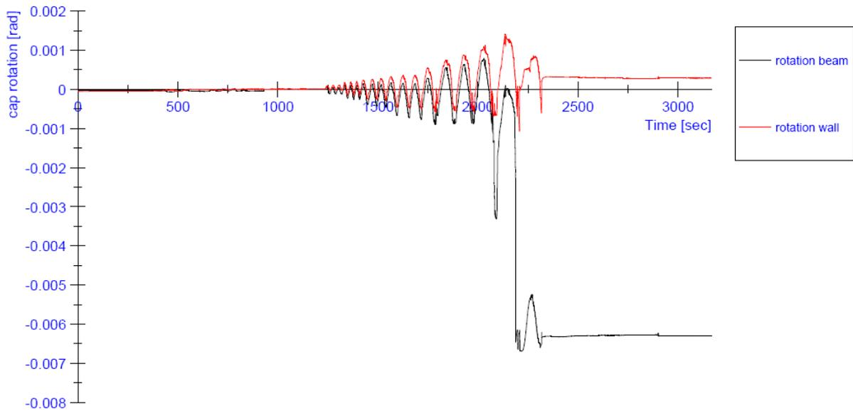
**Figure 77:** Progress of the in-plane rotation at the top of the wall during the test on specimen CS05
