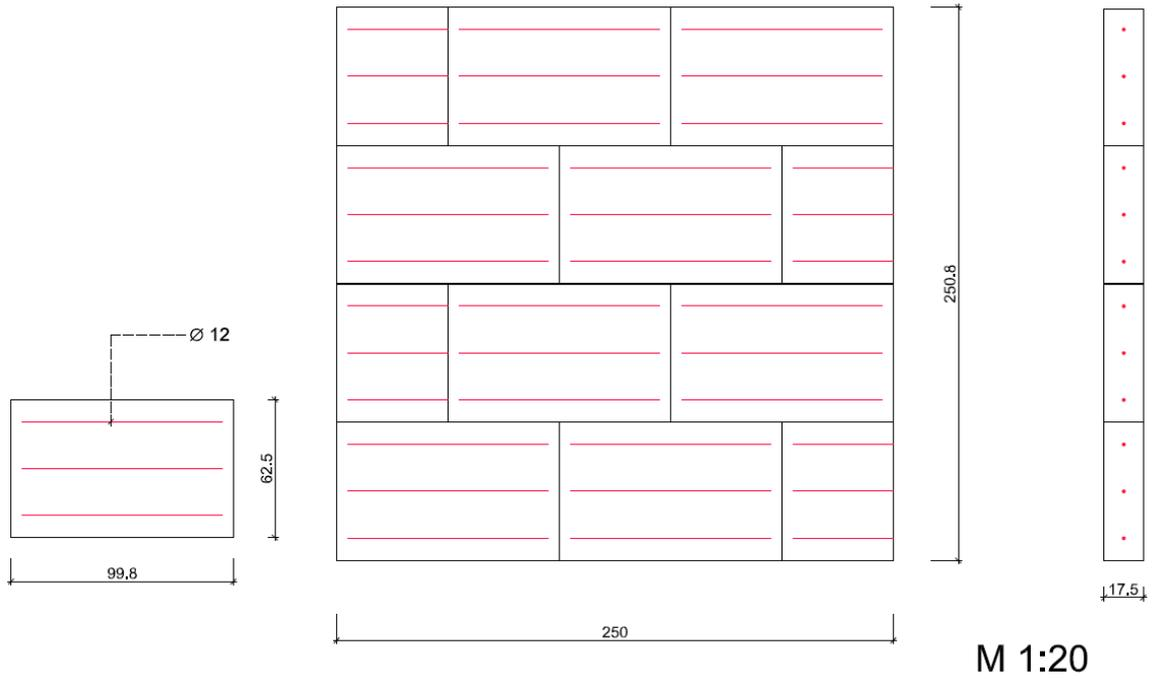
**Figure 66:** Dimension of the test specimen CS05
