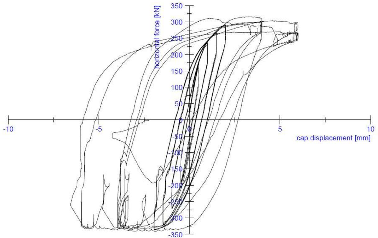
**Figure 71:** Load-displacement curve (hysteresis) of the test on specimen CS05
