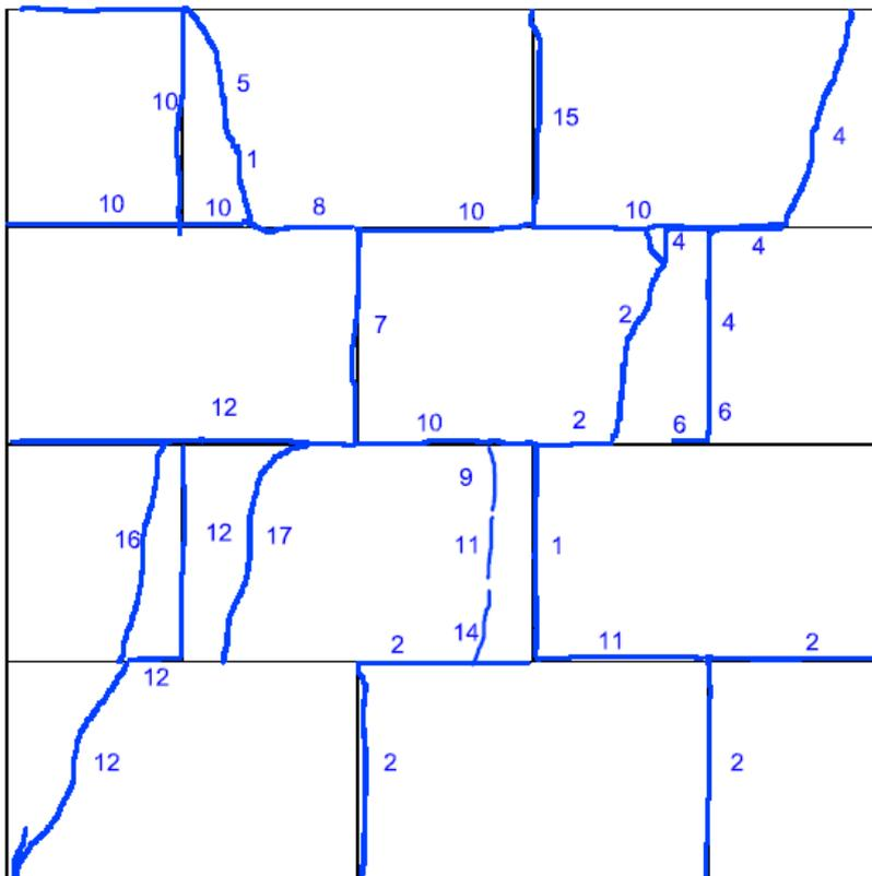
Figure 45: Crack pattern of the test specimen CS03
