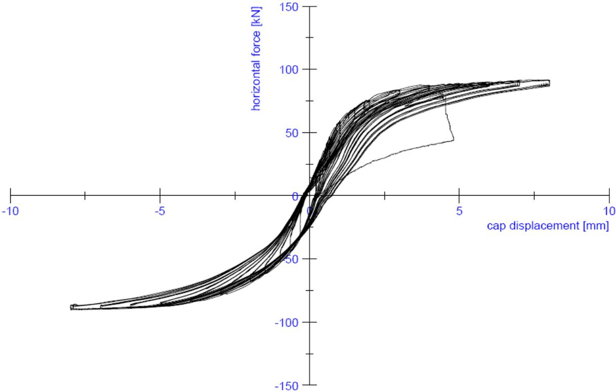
Figure 59: Load-displacement curve (hysteresis) of the test on specimen CS04
