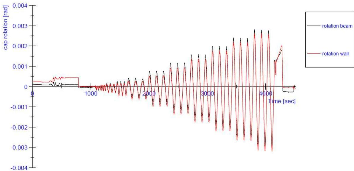
**Figure 65:** Progress of the in-plane rotation at the top of the wall during the test on specimen CS04
