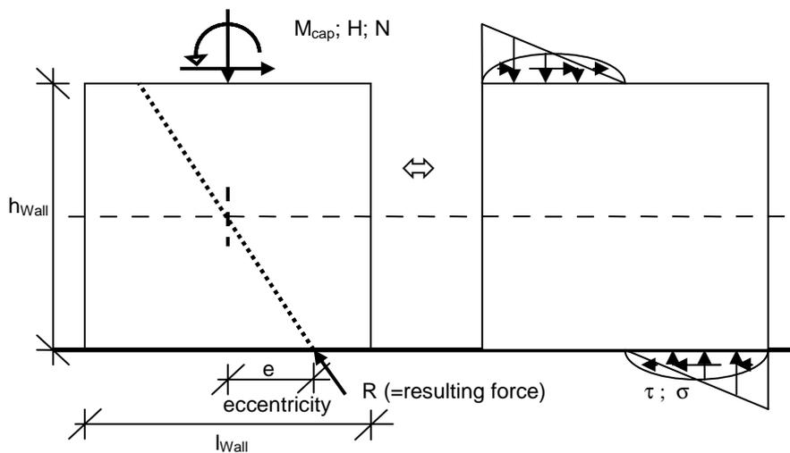
**Figure 6:** Idealized load and stress state at a single wall according to the defined boundary conditions [Deliverable 6.3]
