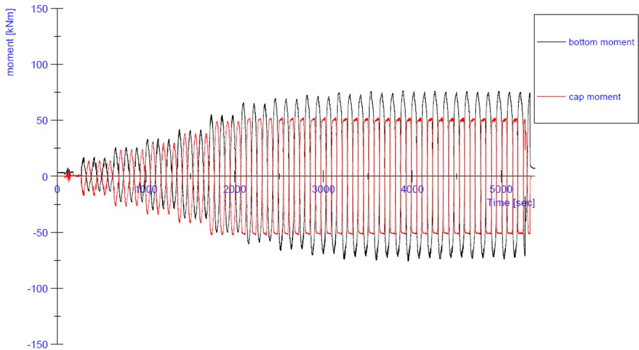
**Figure 112:** Progress of the in-plane bending moments at the top and at the bottom of the wall during the test on specimen Clay01
