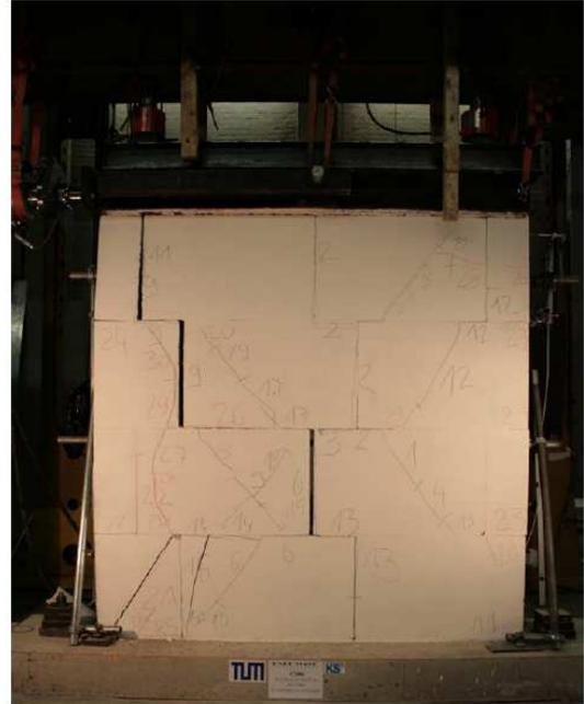
Figure 82: Crack pattern of the test specimen CS06
