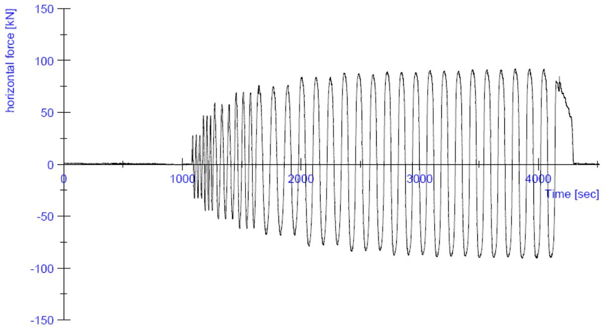
**Figure 61:** Progress of the horizontal force H during the test on specimen CS04
