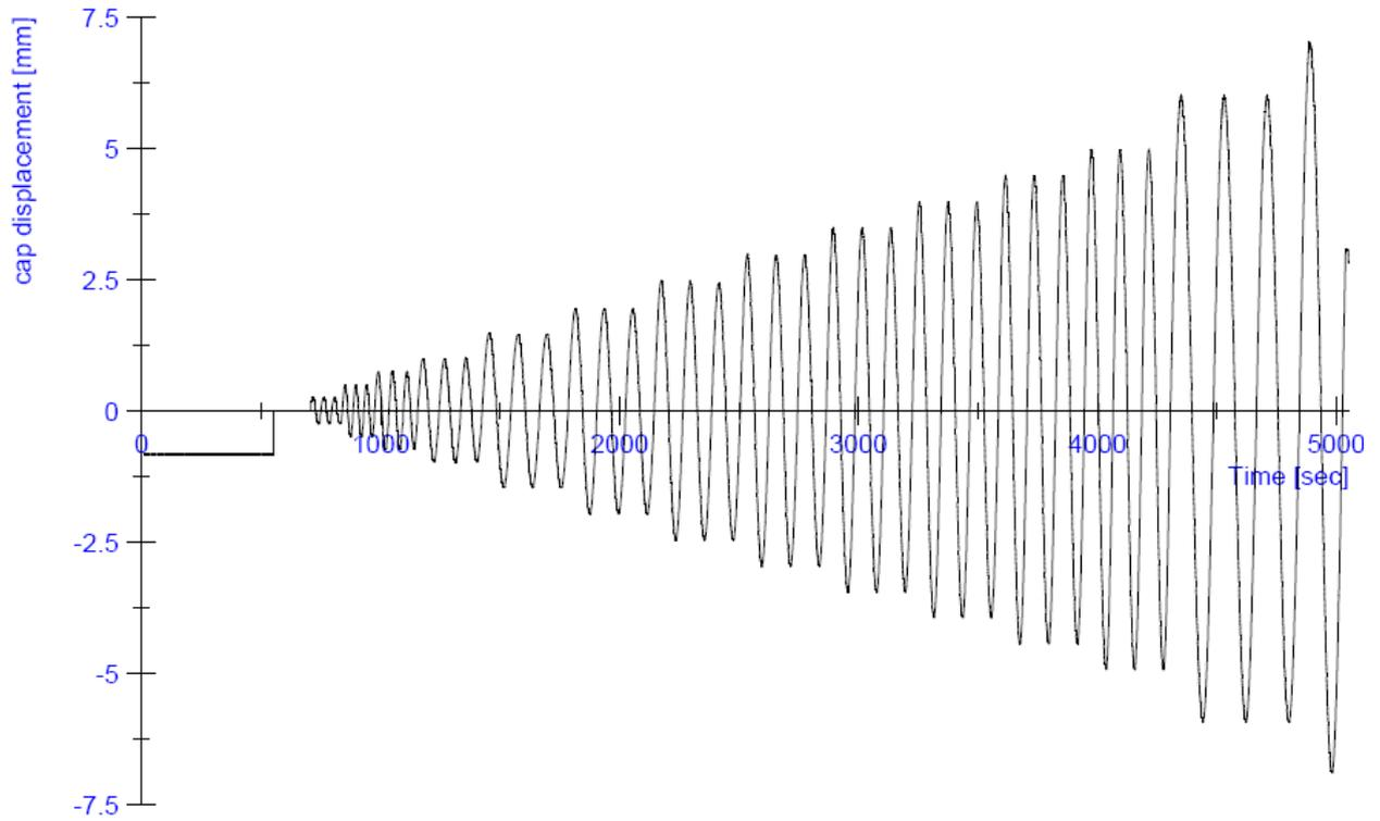
**Figure 98:** Progress of the horizontal displacement during the test on specimen CS07
