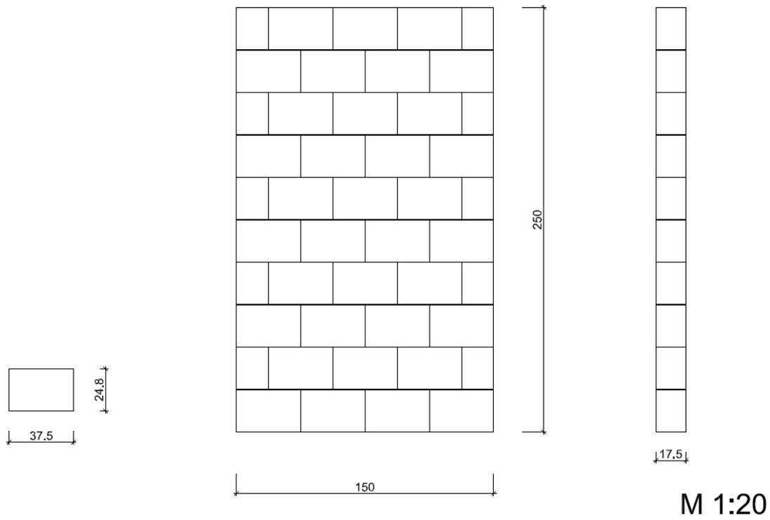
**Figure 102:** Dimension of the test specimen Clay01
