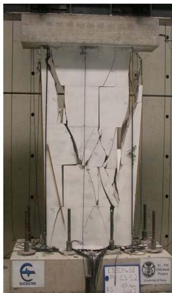
Figure 27 Wall CS12. Confined (1+1 $\phi$ 16), double fixed, l=1.25 m,  $\sigma_v=2.0$  MPa
