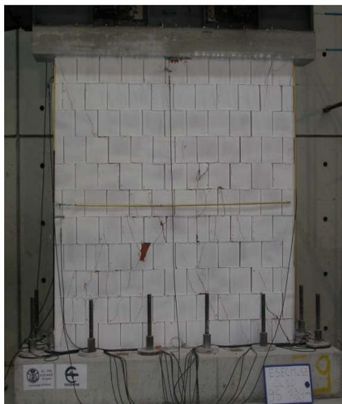
Figure 39 Wall CL10. T+G unit, Thin layer bedjoints, unfilled headjoints  $l=2.50$  m,  $\sigma_v=0.68$  MPa
