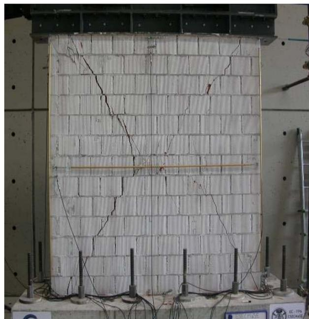
Figure 34 Wall CL05. Traditional unit, G.P. bedjoints and headjoints  $l=2.50$  m,  $\sigma_v=0.68$  MPa
