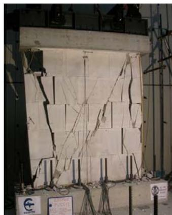
Figure 28 Wall CS13. Confined (1+1 $\phi$ 16), double fixed,  $l=2.50$  m,  $\sigma_v=1.0$  MPa
