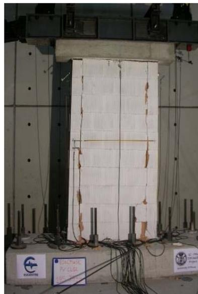
Figure 31 Wall CL02. Confined (1+1 $\phi$ 16), cantilever,  $l=1.50$  m,  $\sigma_v=0.33$  MPa
