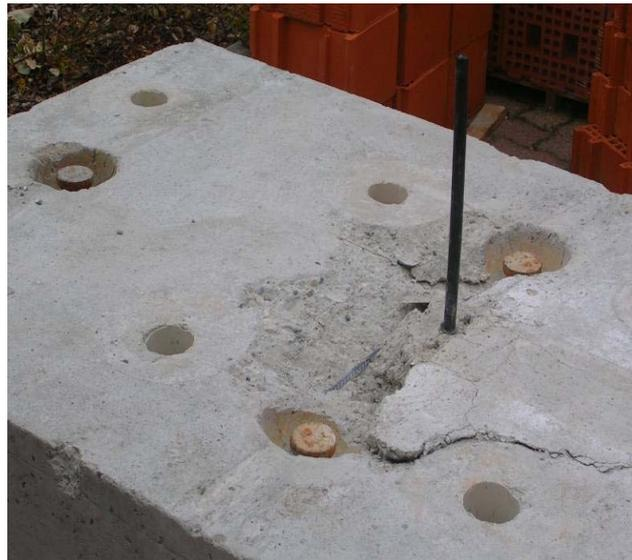
Figure 29 Wall CS14. Post-tensioned, cantilever,  $l=1.25$  m,  $\sigma_v=1.0$  (+1.0) MPa
