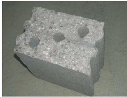
Figure 14. Lightweight aerated concrete T+G units used in walls LAC01, LAC03 ( $l \times t \times h = 247 \times 175 \times 238$  mm) and LAC02, LAC04 ( $l \times t \times h = 247 \times 175 \times 248$  mm)
