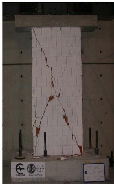
Figure 36 Wall CL07. T+G unit, G.P. bedjoints, unfilled headjoints  $l=1.25$  m,  $\sigma_v=0.50$  MPa
