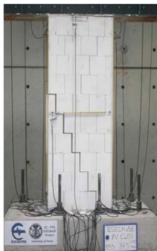
Figure 32 Wall CL03. Unreinforced, double fixed,  $l=1.00$  m,  $\sigma_v=0.14$  MPa
