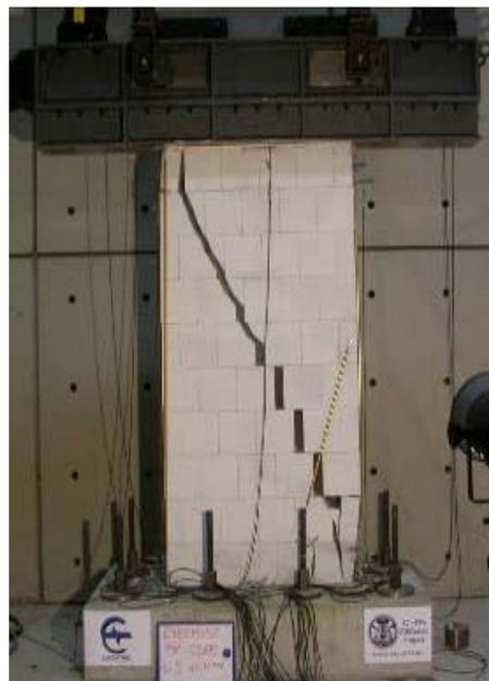
Figure 20 Wall CS05. Double fixed,  $l=1.25$  m,  $\sigma_v=1.0$  MPa, filled head joints
