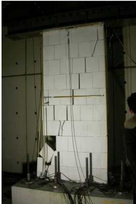
Figure 16 Wall CS01. Double fixed,  $l=1.25$  m,  $\sigma_v=1.0$  MPa
