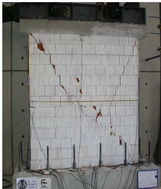
Figure 37 Wall CL08. T+G unit, G.P. bedjoints, unfilled headjoints  $l=2.50$  m,  $\sigma_v=0.68$  MPa
