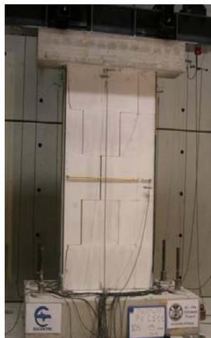
Figure 26 Wall CS11. Confined (1+1 $\phi$ 16), double fixed, l=1.25 m,  $\sigma_v=0.5$  MPa
