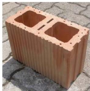
Figure 8. 175 mm thick hollow clay unit T+G used in the walls CL01 and CL02
