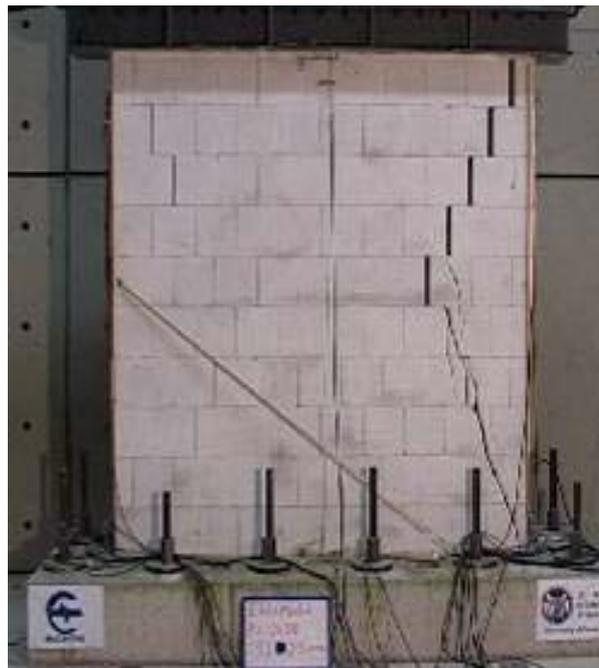
Figure 23 Wall CS08. Cantilever,  $l=2.50$  m,  $\sigma_v=1.0$  MPa
