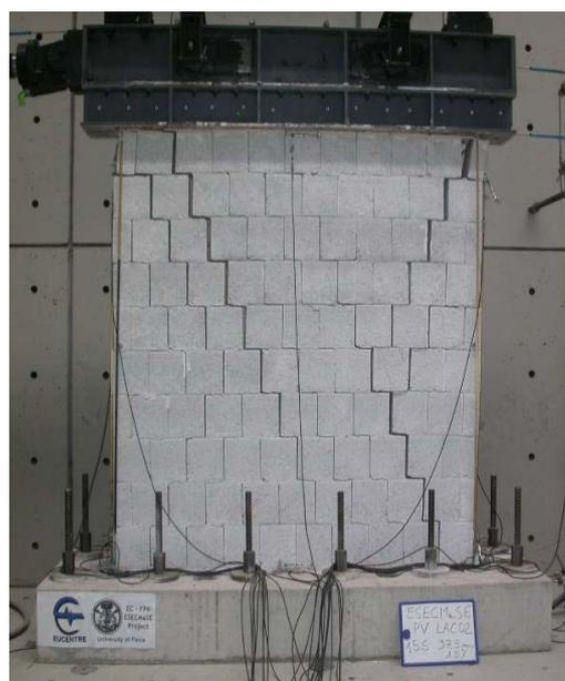
Figure 41 Wall LAC02. Thin layer bedjoints, unfilled headjoints,  $l=2.50$  m,  $\sigma_v=0.50$  MPa
