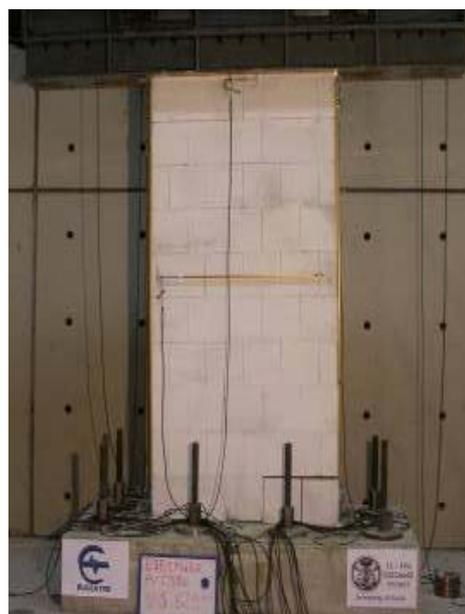
Figure 21 Wall CS06. Cantilever,  $l=1.25$  m,  $\sigma_v=1.0$  MPa
