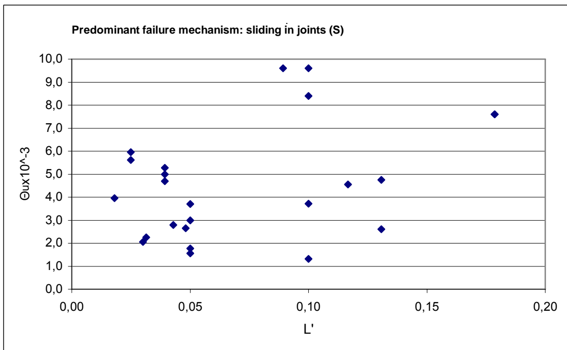
Fig. 5c: Interstorey drift angle as a function of L' for specimens with predominant sliding in joints
