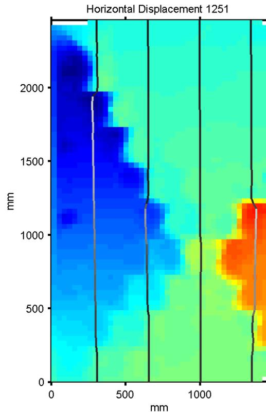
Figure 32 - Residual horizontal displacement field after test at 0.12g
