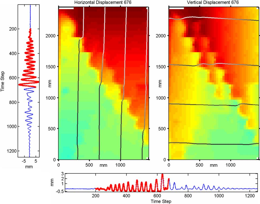
Figure 31 Primary diagonal stepwise crack fully developed
