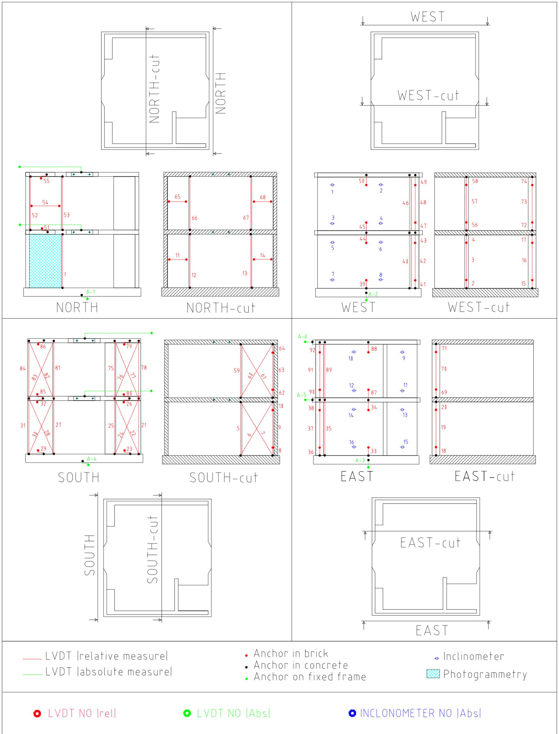
Figure 5: Instrumentation of the clay specimen
