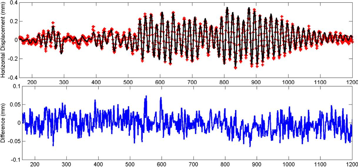
Figure 24 – H1 (black), optical signal (red crosses) and difference (blue) for 0.02g
