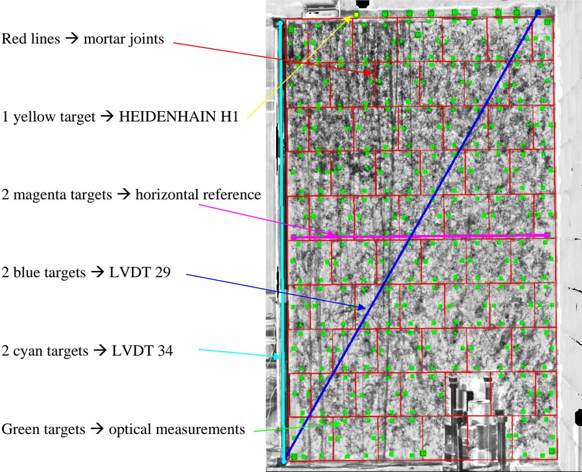
Figure 23- The main shear wall after segmentation and segregation
