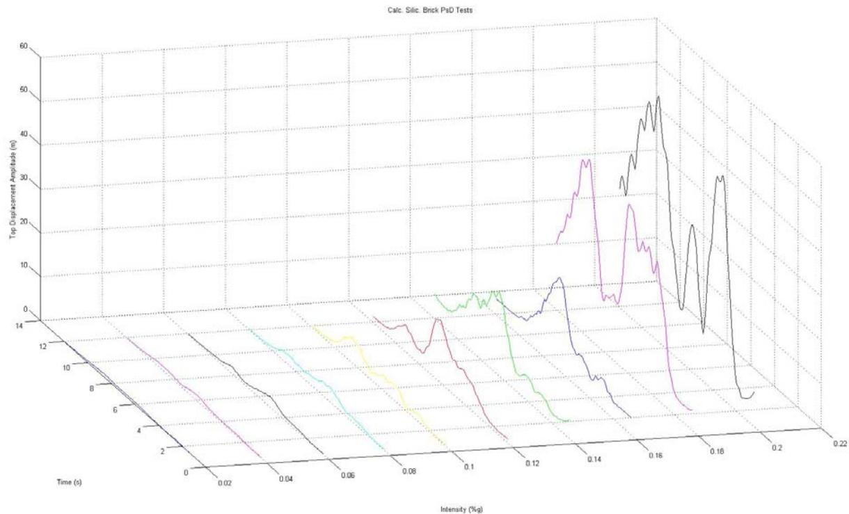
Figure 10 Top displacement amplitudes for the calcium silicate specimen
