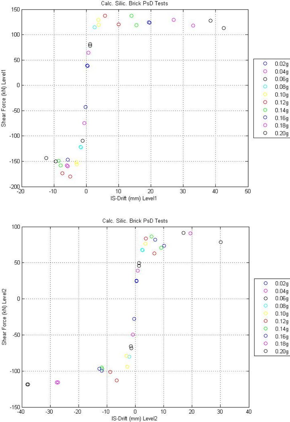
Figure 12: Envelope of the shear drift curves for the calcium silicate specimen
