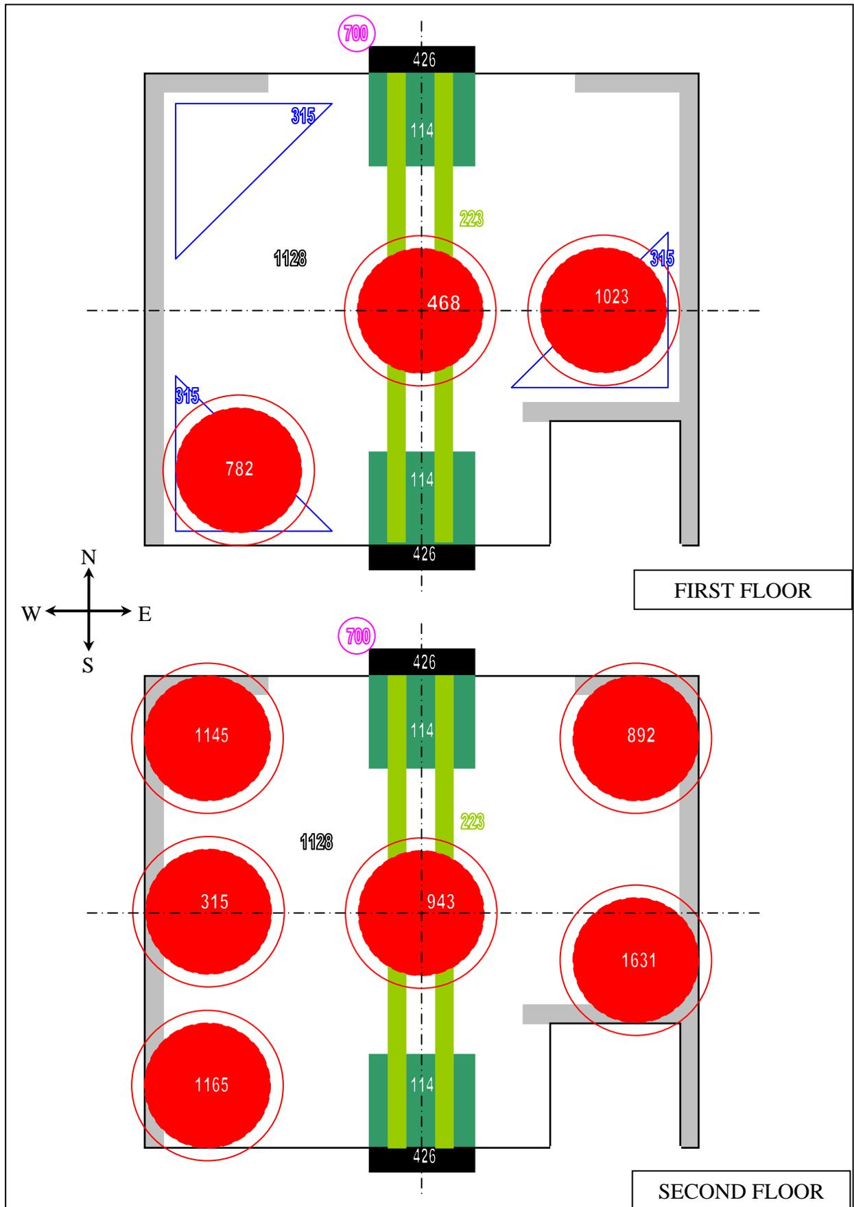
Figure 2– Distribution of the water tanks on the calcium silicate specimen
