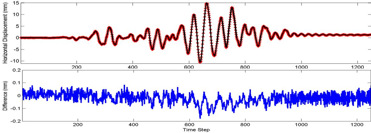
Figure 25 – H1 (black), optical signal (red crosses) and difference (blue) for 0.16g
