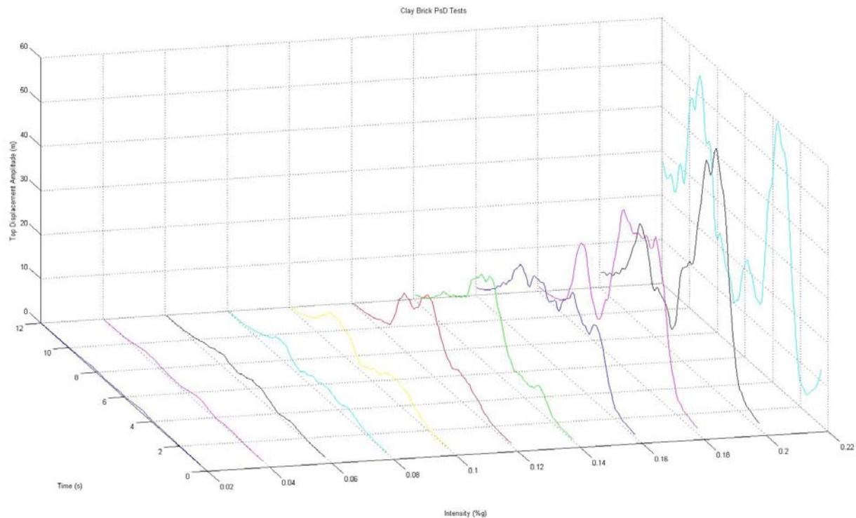
Figure 19- Top displacement amplitudes for the clay specimen
