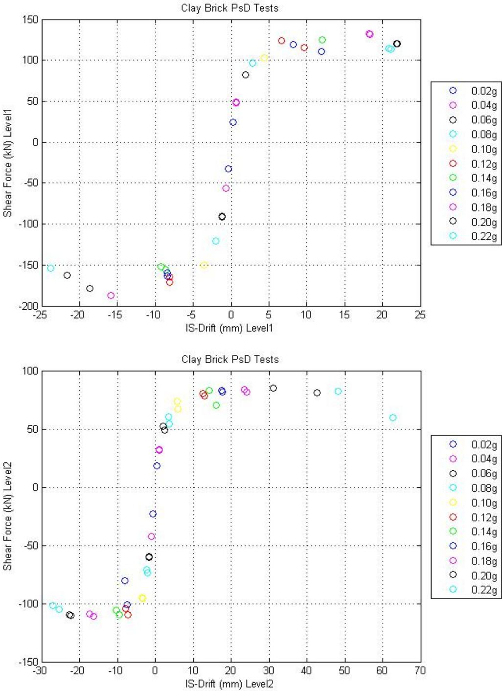
Figure 21: Envelope of the shear drift curves for the brick specimen
