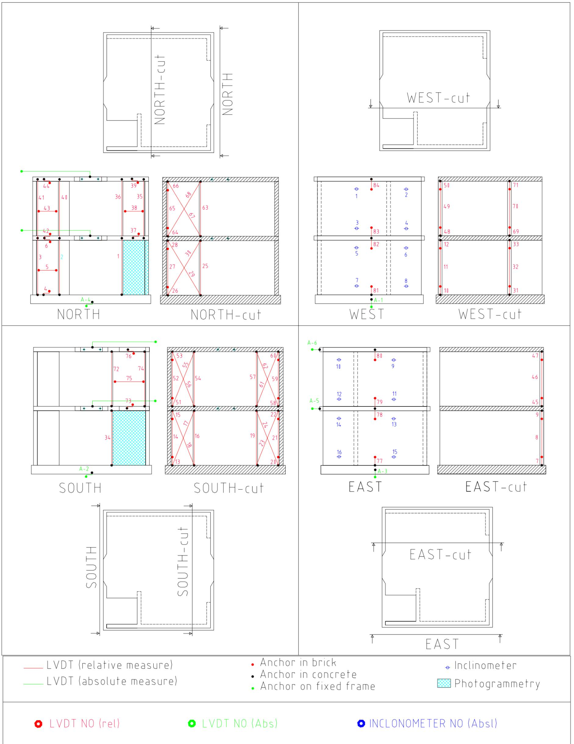
Figure 4: Instrumentation of the calcium silicate specimen
