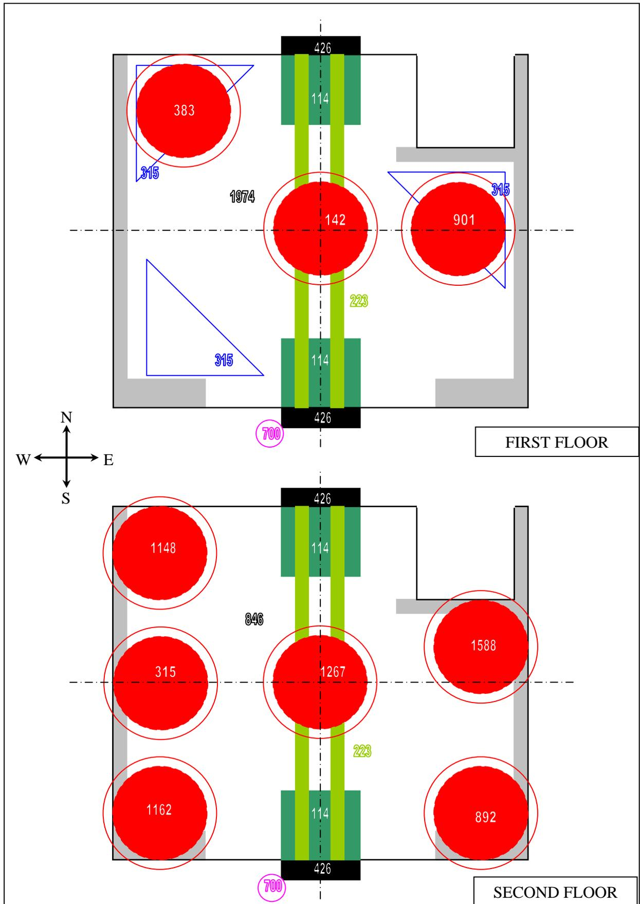
Figure 3– Distribution of the water tanks on the clay specimen
