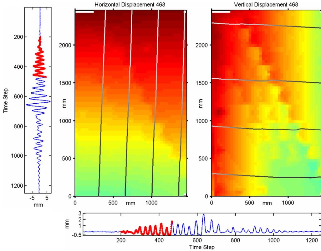
Figure 29 - Primary stepwise crack initiation along the compressed diagonal
