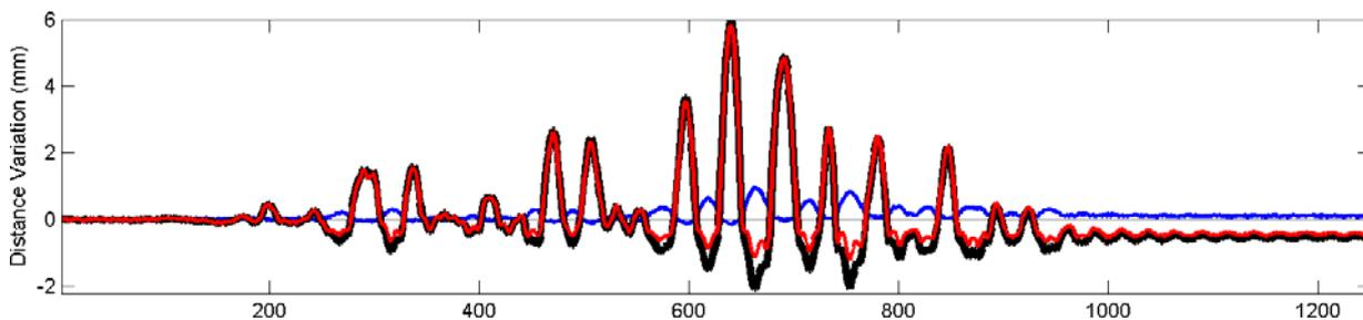
Figure 27 – LVDT 29 (black), optical signal (red) and difference (blue) for 0.16g
