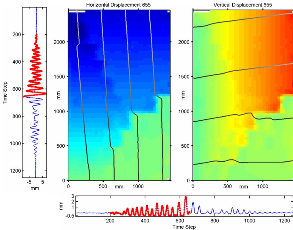
Figure 30 - Secondary stepwise crack at mid-height
