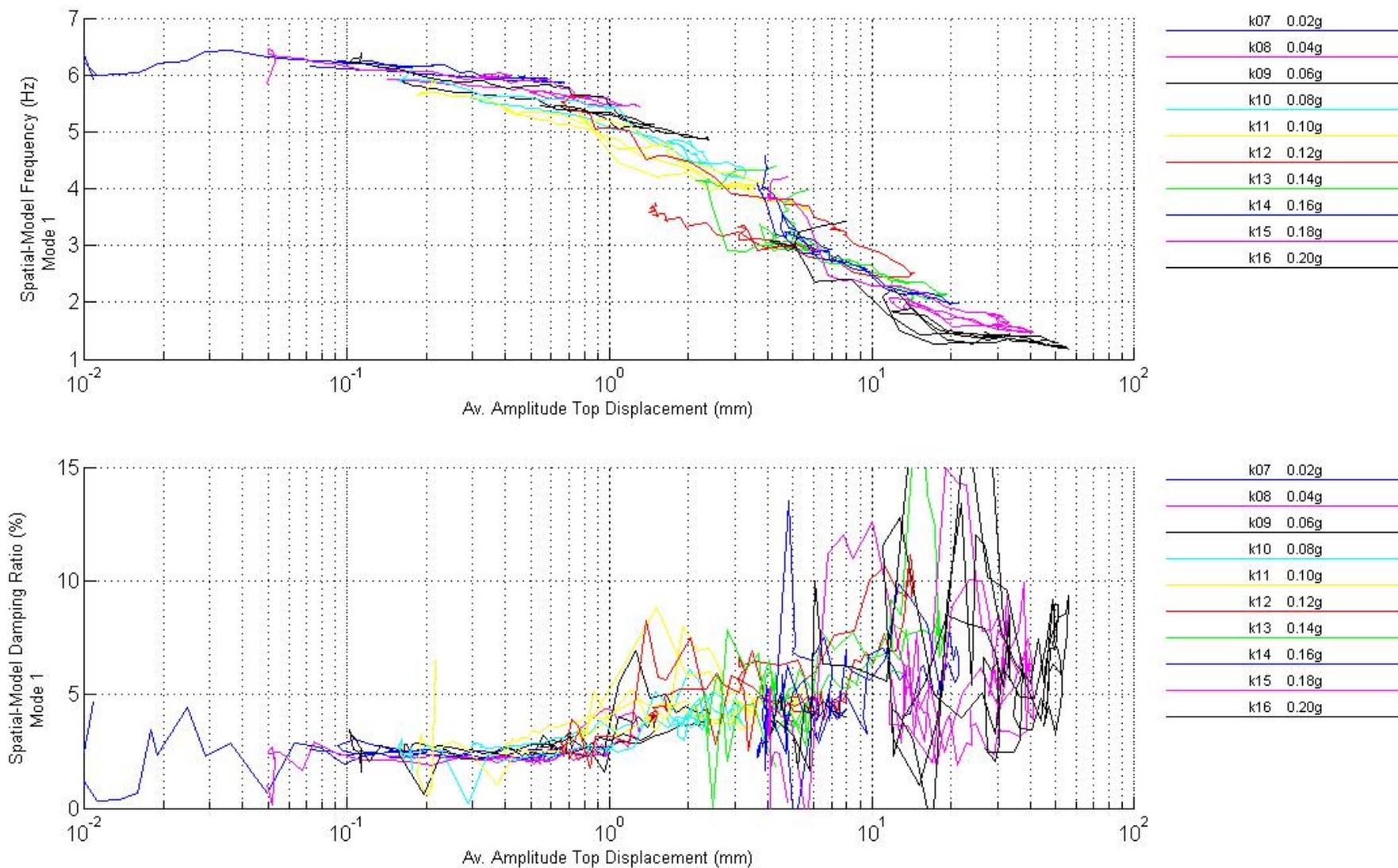
Figure 11: Evolution of the 1<sup>st</sup> frequency and damping against the top displacement amplitude
