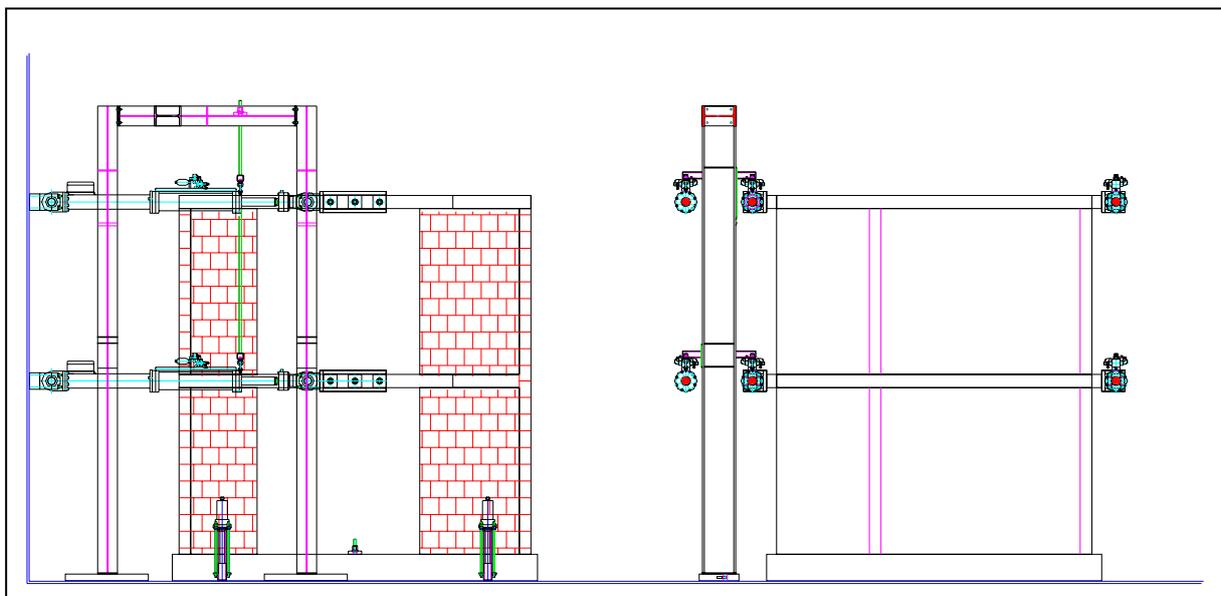
Figure 1– Balancing system for the actuators
