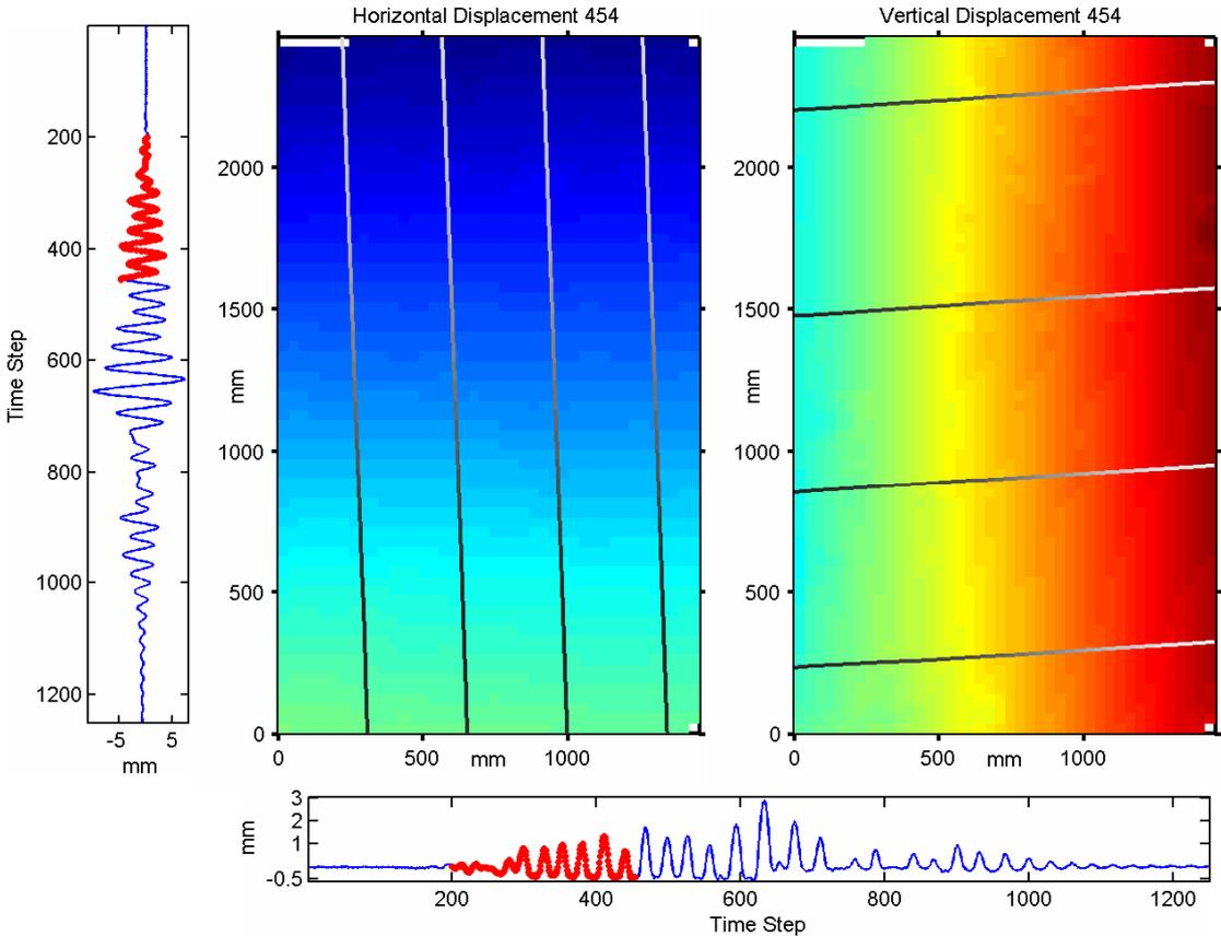
Figure 28 - Pure rocking behaviour of the wall
