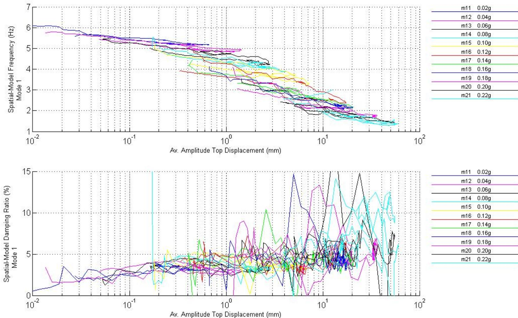
Figure 20: Evolution of the 1<sup>st</sup> frequency and damping against the top displacement amplitude
